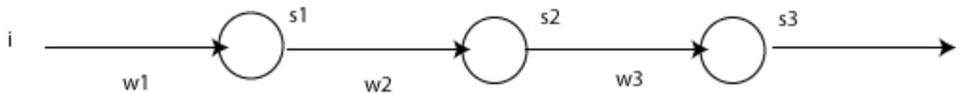
Note that the input to the net is  $i$  and the outputs of the sigmoid units are  $s_1, s_2,$  and  $s_3$ .
