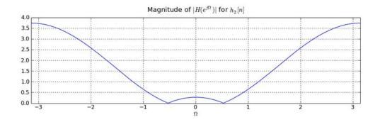
Note, the only nonzero values of unit sample response for  $H_2$  are :  $h_2[0] = 1$ ,  $h_2[1] = -sqrt(3)$ ,  $h_2[2] = 1$ .
