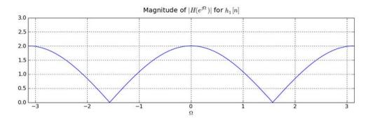
Note: the only nonzero values of unit sample response for  $H_1$  are :  $h_1[0] = 1$ ,  $h_1[1]=0$ ,  $h_1[2]=1$ .
