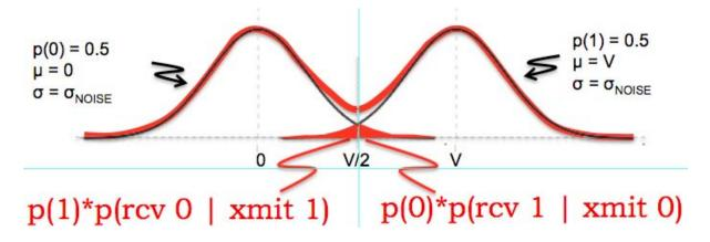
so the bit-error rate is given by 0.5\*erfc(V/(sqrt(8)\*sigma)). Note that sigma = sqrt(N0/2) using the definition of N0. This formula is related to the  $0.5*sqrt(E_s/N0)$  from Chapter 5 and the lecture;  $E_s$  in our case is V\*V/4.
