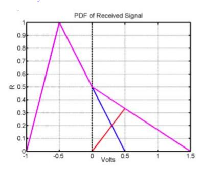
d. What digitization threshold voltage would minimize the bit error rate?
