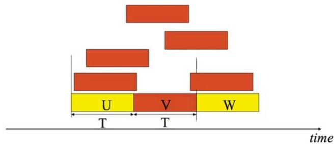
Figure 15-7: Each packet is  $T$  slots long. Packet transmissions begin at a slot boundary. In this picture, every packet except  $U$  and  $W$  collide with  $V$ . Given packet  $V$ , any other packet sent in any one of  $2T - 1$  slots—the  $T$  slots of  $V$  as well as the  $T - 1$  slots immediately preceding  $V$ 's transmission—collide with  $V$ .
