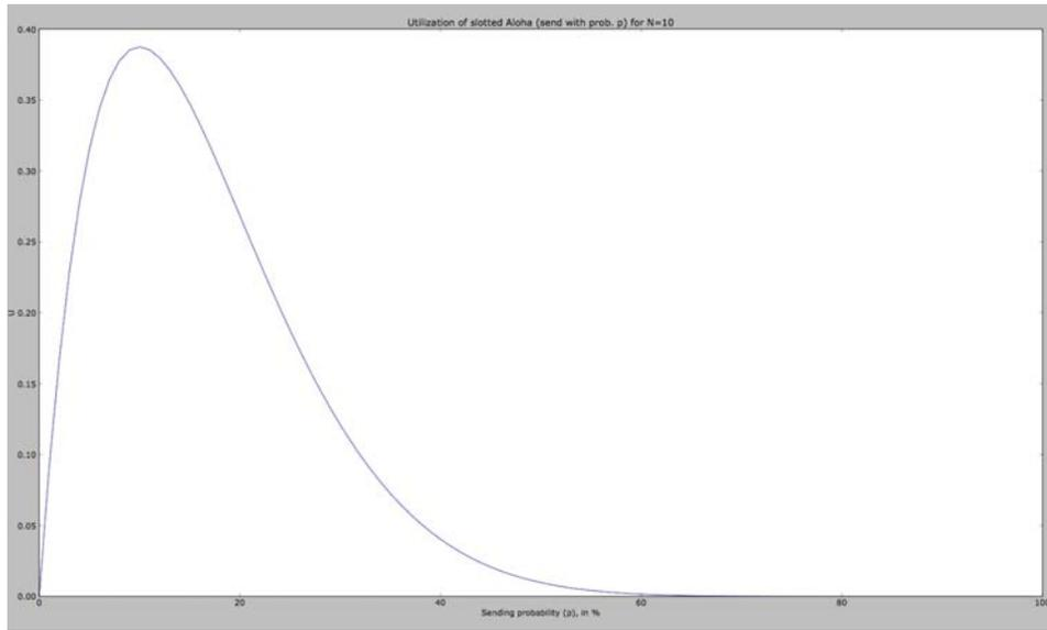
**Figure 15-3:** The utilization of slotted Aloha as a function of  $p$  for  $N = 10$ . The maximum occurs at  $p = 1/N$  and the maximum utilization is  $U = (1 - \frac{1}{N})^{N-1}$ . As  $N \rightarrow \infty$ ,  $U \rightarrow \frac{1}{e} \approx 37\%$ .  $N$  doesn't have to be particularly large for the  $1/e$  approximation to be close—for instance, when  $N = 10$ , the maximum utilization is 0.387.
