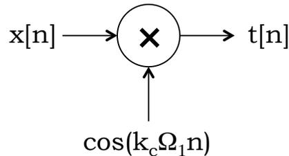
**Figure 14-3: Modulation involved “mixing”, or multiplying, the input signal  $x[n]$  with a carrier signal  $\cos(\Omega_c n) = \cos(k_c\Omega_1 n)$  here) to produce  $t[n]$ , the transmitted signal.**
