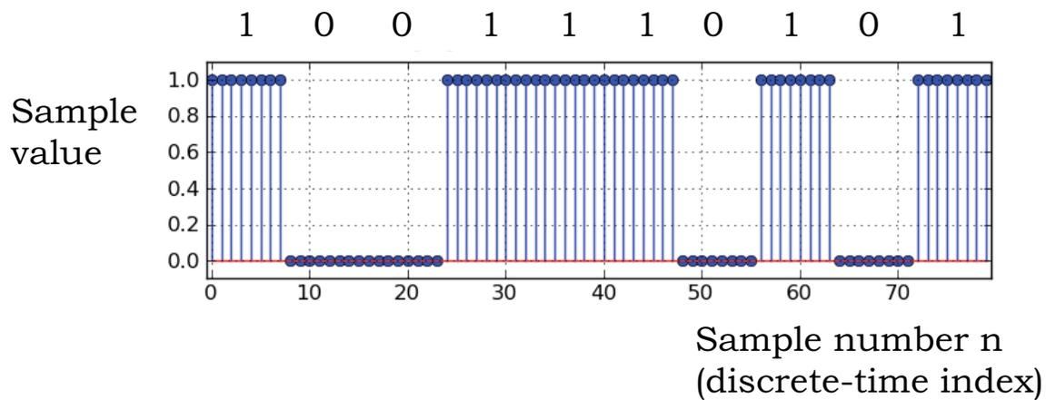
Figure 10-2: Digitized samples of the baseband signal.
