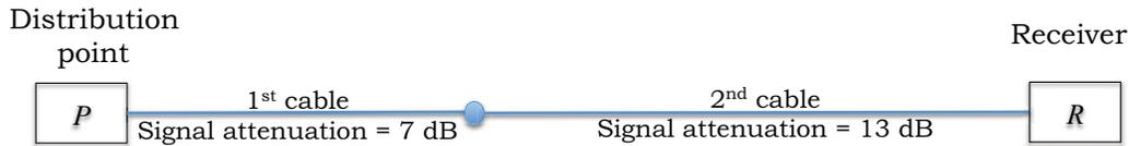
The first cable attenuates (i.e., reduces) the signal power by 7 dB. The second cable attenuates the signal power by an **additional** 13 dB. Calculate  $\frac{P}{R}$  as a numeric ratio.
