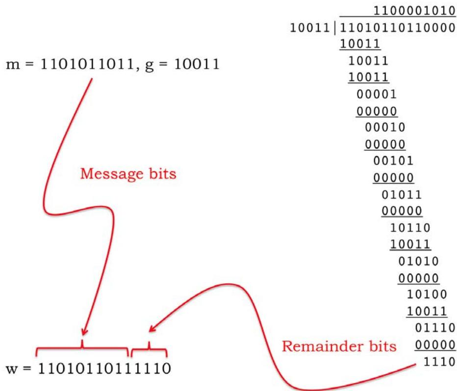
Figure 6-3: CRC computations using “long division”.
