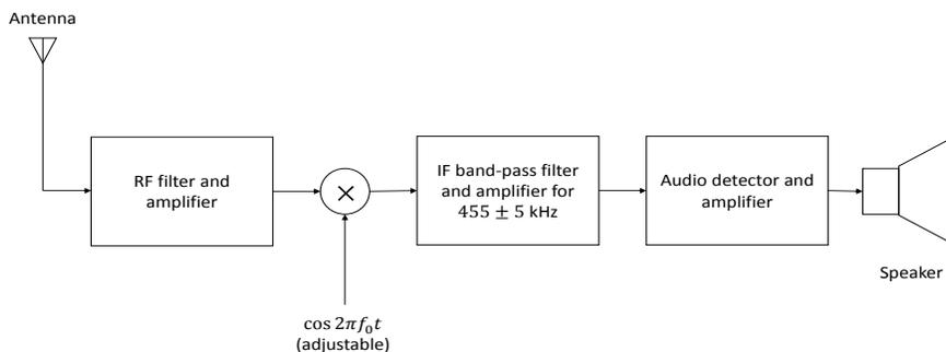
Figure 5: Structure of a typical radio receiver.
