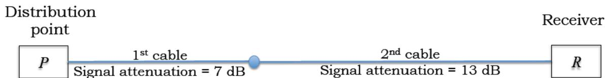
The first cable attenuates (i.e., reduces) the signal power by 7 dB. The second cable attenuates the signal power by an additional 13 dB. Calculate P/R as a numeric ratio.
