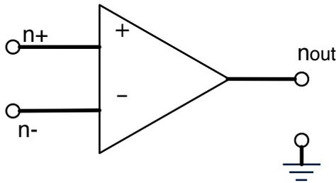
The simplified behavioral model is that the op-amp adjusts  $v_{out}$  in order to try to maintain the constraint that  $v_+ \approx v_-$  and that no current flows in to  $n_+$  or  $n_-$ . In what follows we will assume that the op-amp enforces  $v_+ = v_-$ .
