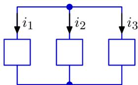
There are two nodes, each indicated by a dot. In an electrical circuit nodes can be thought of as wires<sup>39</sup> that connect a component.
