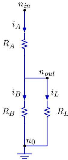
We've shown an additional "load" on the circuit at  $V_{out}$  with a resistor  $R_L$  standing for whatever resistance that additional load might offer to the ground node  $n_0$ . This changes matters considerably.
