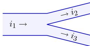
Let  $i_1$  represent the flow into the branching point and  $i_2$  and  $i_3$  represent the flows out of it. Assume that  $i_1$ ,  $i_2$ , and  $i_3$  have the units of volume per unit time (e.g.,  $\text{m}^3/\text{s}$ ).
