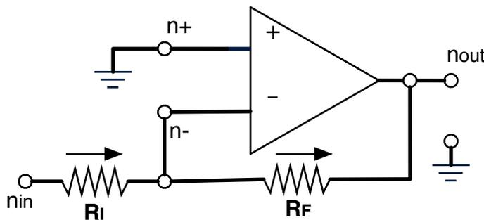
The difference is that the + terminal of the op-amp is connected to ground, and we're thinking of the path through the resistors as the terminal of the resulting circuit. Let's figure out the relationship between  $v_{in}$  and  $v_{out}$  for this one. The circuit constraints tell us that
