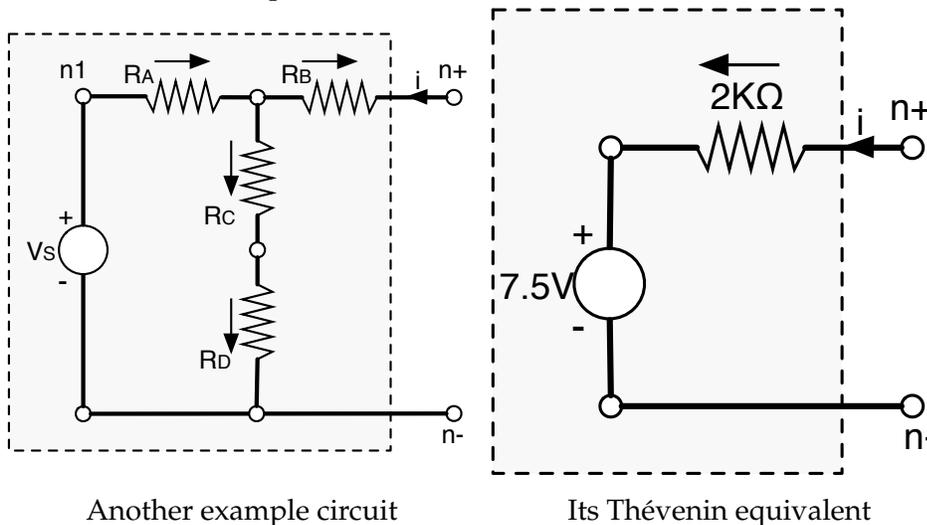
It's a bit more hassle than the previous one, but you can write down the equations to describe the constituents and KCL constraints, as before. If we let  $R_A = 2K\Omega$ ,  $R_B = R_C = R_D = 1K\Omega$ , and  $V_s = 15V$ , then we can solve for  $V_{th} = 7.5V$  and  $R_{th} = 2K\Omega$ . So, it is indistinguishable by current and voltage from the circuit shown in the equivalent circuit.
