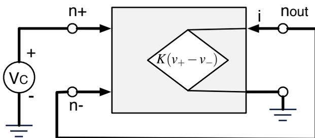
Note that we have connected a wire from the output,  $n_{out}$ , to the negative input,  $n_-$ , and so those constitute one node with a single voltage, which we call  $v_{out}$ . We can write down the equations:
