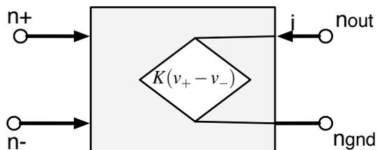
A model of the constraint that an op-amp exerts on the circuit it is connected to relates the voltages at its four terminals in this way:
