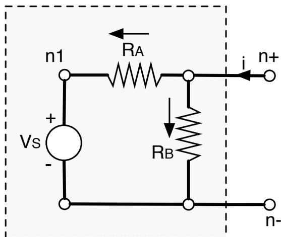
The first step is to compute the open-circuit voltage. This just means figuring out the difference between the voltage at nodes  $n_+$  and  $n_-$ , under the assumption that the current  $i = 0$ . An easy way to do this is to set  $n_-$  as ground and then find the node voltage at  $n_+$ . Let's write down the equations:
