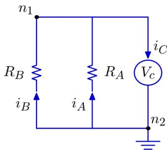
we have a simple circuit with two resistors in parallel. Even though there are a lot of wires being connected together, there are really only two nodes: places where multiple components are connected. Let's write down the equations governing this system.
