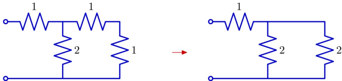
Combine rightmost parallel resistors, then the resulting series.
