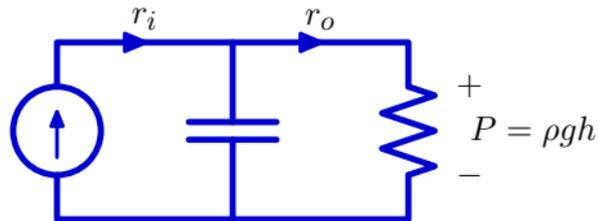
Flow of water into and out of tank are represented as “through” variables  $r_i$  and  $r_o$ , respectively. Hydraulic pressure at bottom of tank is represented by the “across” variable  $P = \rho gh$ .
