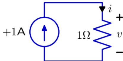
The current source determines the current through the resistor,  $i = 1\text{A}$ , so the voltage across the resistor is  $v = iR = 1 \times 1 = 1\text{V}$ .
