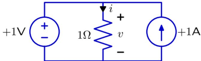
If all of the current from current source flowed through the resistor, then it would generate  $1\text{V}$  across the resistor.
