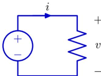
The voltage source generates a voltage  $v$  across the resistor and a current  $i$  through the resistor.
