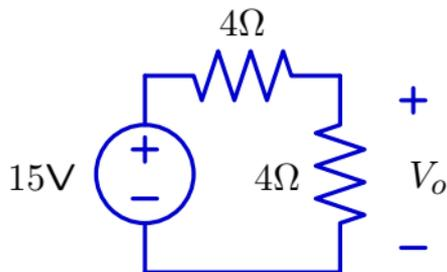
Now apply the voltage divider relation:  $V_o = \frac{4\Omega}{4\Omega + 4\Omega} \times 15\text{V} = 7.5\text{V}$ .
