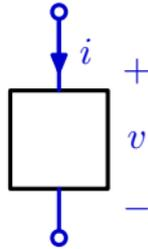
A one-port has two terminals. Current enters one terminal (+) and exits the other (-), producing a voltage ( $v$ ) across the terminals.
