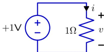
The voltage source determines the voltage across the resistor,  $v = 1\text{V}$ , so the current through the resistor is  $i = v/R = 1/1 = 1\text{A}$ .
