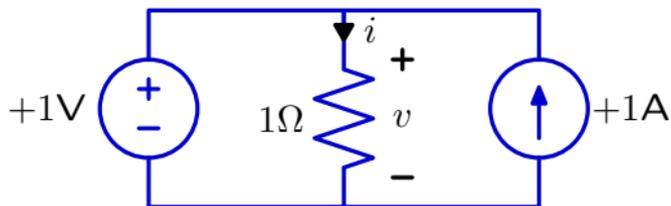
The voltage source forces the voltage across the resistor to be  $1\text{V}$ . Therefore, the current through the resistor is  $1\text{V}/1\Omega = 1\text{A}$ .
