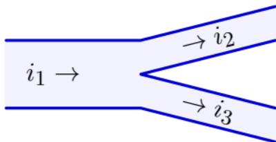
Current  $i_1$  flows into a **node** and two currents  $i_2$  and  $i_3$  flow out:
