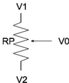
Give an expression (in terms of  $V_1$ ,  $V_2$ , and  $R_P$ ) for the value of  $V_0$  when  $\alpha = 0$ :
