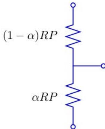
By connecting a potentiometer as shown below we can create a device that converts  $\alpha$  into a voltage  $V_0$ . **All voltages are measured relative to ground.**
