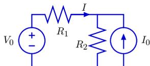
Turning off  $I_0$  (i.e.,  $I_0 = 0$ ) is equivalent to an open circuit.
