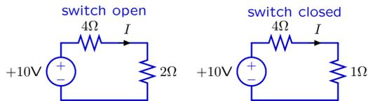
Closing the switch decreases equivalent resistance to right of  $I$ .
