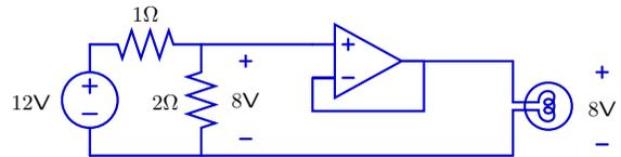
This op-amp circuit produces an output voltage equal to its input voltage (8V) while having no effect on the left part of the circuit.
