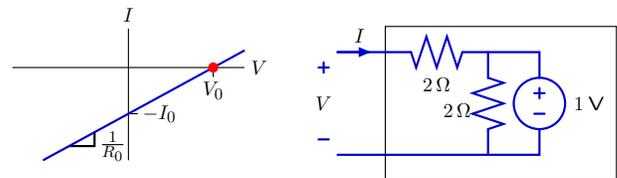
Set  $I = 0$  in the circuit. Then  $V = V_0 = 1V$ .
