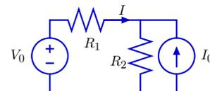
Turning off  $V_0$  (i.e.,  $V_0 = 0$ ) is equivalent to a short circuit.
