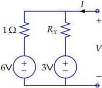
Determine the short-circuit current if  $R_x = 3 \, \mathrm{Ohm} s$ .
