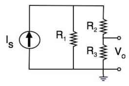
Assume  $R_1 = R_2 = 10$  ohms each,  $R_3 = 5$  Ohms and the current source  $I_S = 10$  amps. What are the values of the Thevenin equivalent voltage and resistance as seen from the  $V_0$  port (where the ground node is treated as the negative terminal of the port)?
