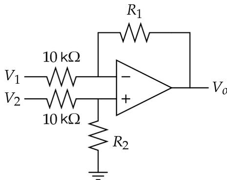
Fill in the values of  $R_1$  and  $R_2$  required to satisfy the equations in the left column of the following table. The values must be non-negative (i.e., in the range  $[0, \infty]$ ). If the equation is impossible to implement with non-negative resistors, then write “impossible” for both resistor values.
