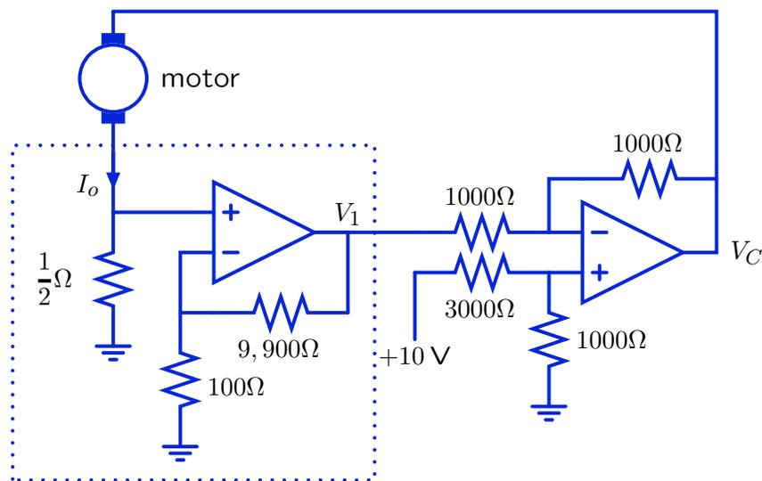
**Part a.** Consider the circuit inside the dotted rectangle. Determine an expression for  $V_1$  as a function of  $I_o$ .
