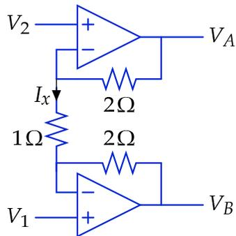
Determine the current  $I_x$  when  $V_1 = 1\text{ V}$  and  $V_2 = 2\text{ V}$ .
