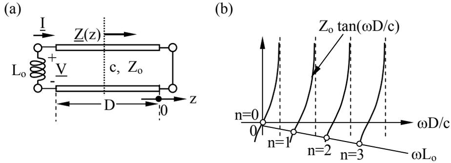
Figure 7.4.2 Inductively loaded TEM transmission line resonator.
