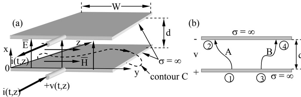
Figure 7.1.1 Parallel-plate TEM transmission line.
