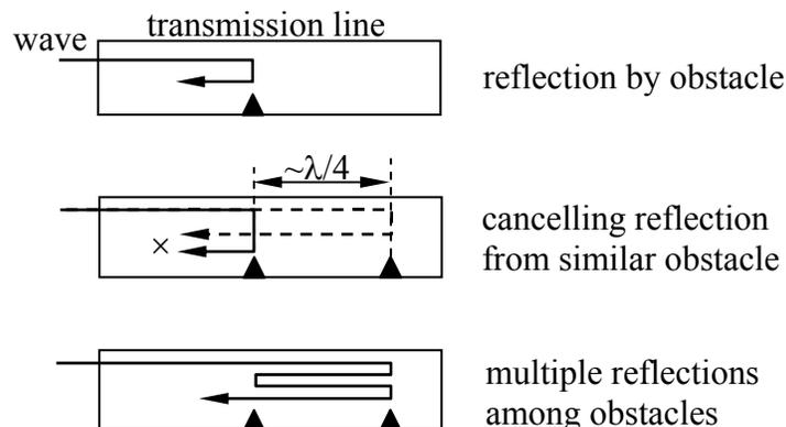
Figure 7.3.1 Cancellation of reflections on transmission lines.
