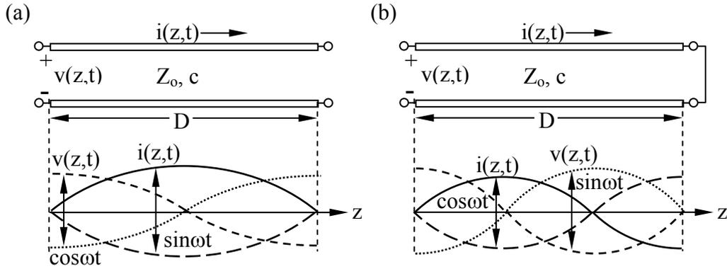
Figure 7.4.1 Voltage and current on TEM resonators.
