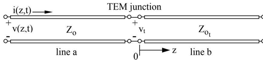
Figure 7.2.1 Junction of two TEM transmission lines.
