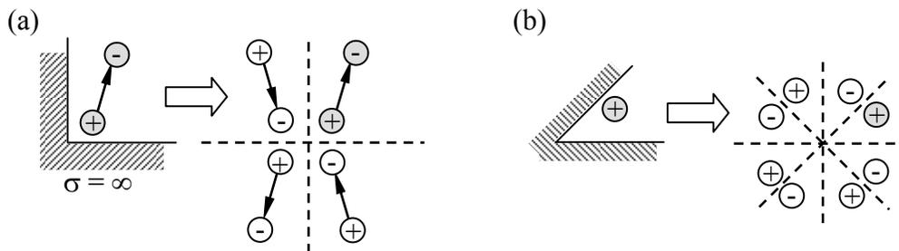
Figure 4.2.4 Image charges and currents for intersecting conductors.
