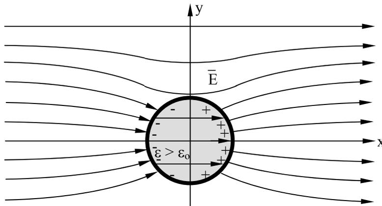
Figure 4.5.2 Electric fields perpendicular to a dielectric cylinder.
