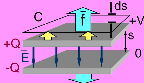
The static pressure  $P_e$  of the electric field on the upper plate is the same with a battery attached:
