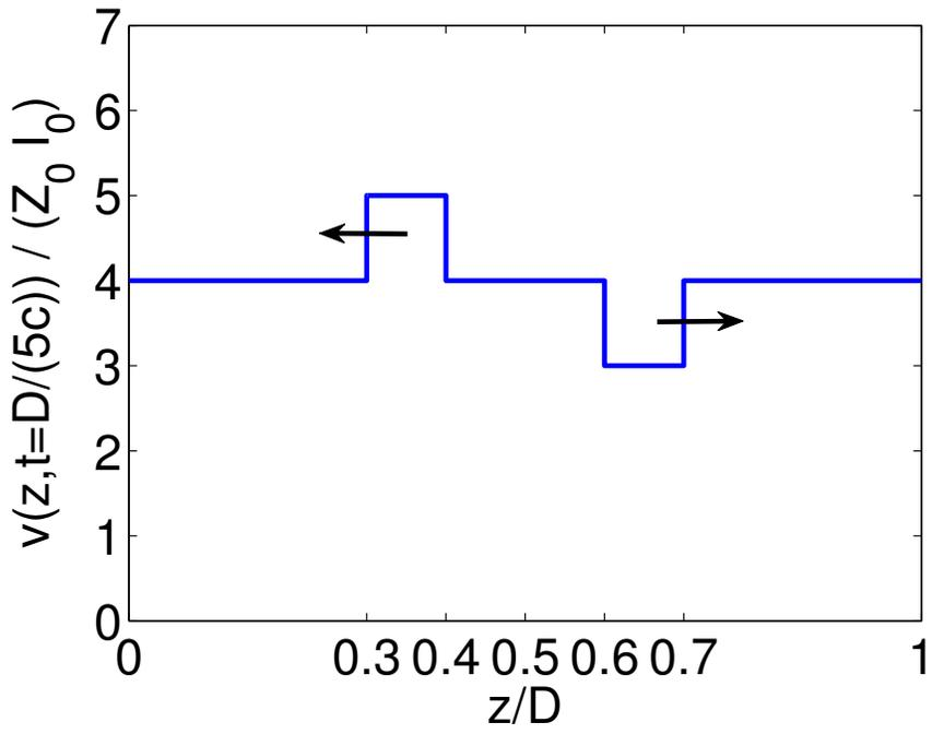
Figure 6.7: Voltage distribution on the line at time,  $t = D/(5c)$ , after the switch was initially opened.
