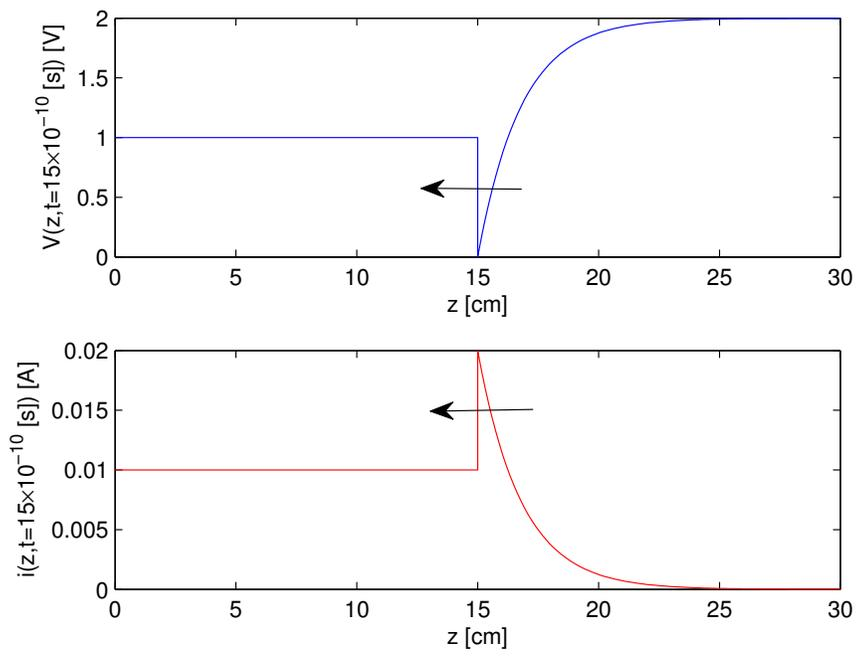
Figure 6.2: Current and voltage distribution at  $3\ell/(2c)$  for capacitive load with  $C = 2 \times 10^{-12}$  F.
