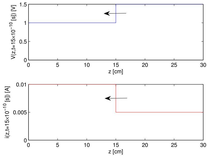
Figure 6.1: Current and voltage distribution at  $3\ell/(2c)$  for  $300 \Omega$  load.
