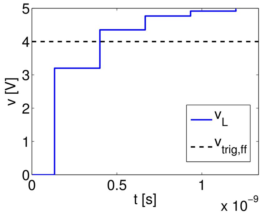
Figure 6.5: Load voltage trace. Triggering occurs when load voltage exceeds flip-flop trigger voltage (here,  $4 \times 10^{-10}$  [s]).
