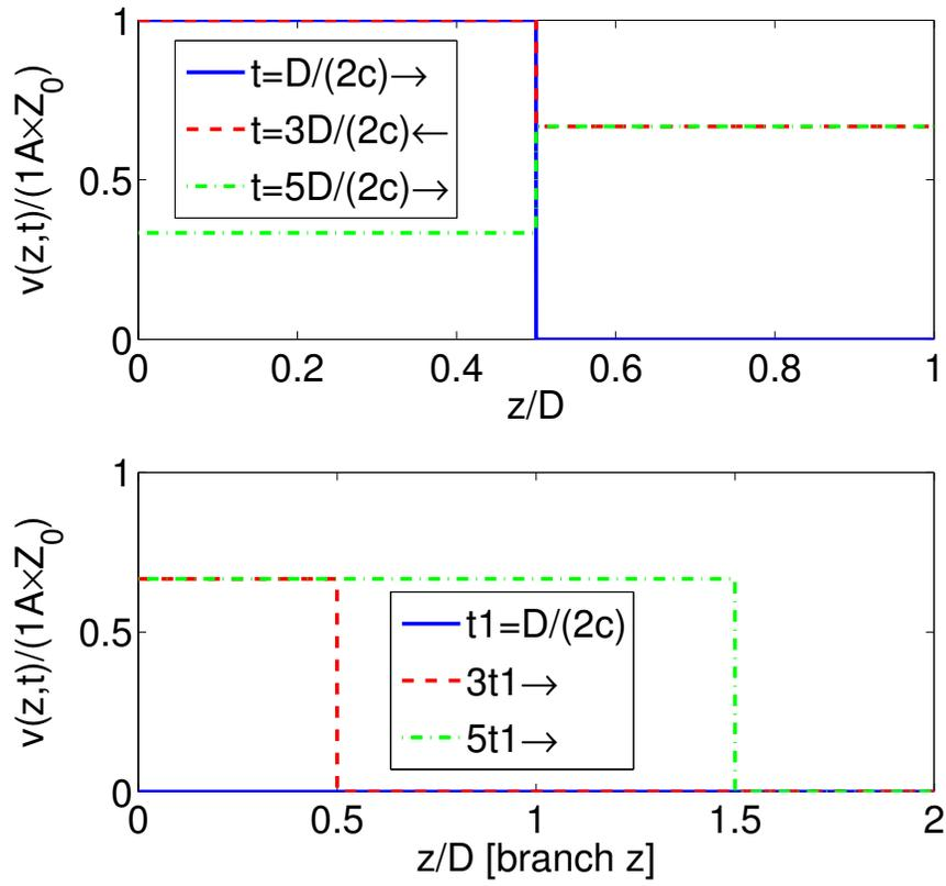
Figure 6.6: Voltage distribution on the primary (top) and branch (bottom) lines.
