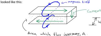
The inductance for this ensemble was  $L = \mu A/W$ , where A is the area looking into the page, and W is the depth into the page. The larger the loop-enclosed area through which flux cross, the larger the inductance. The further the flux lines travel through the structure, the greater the magnetic reluctance, the weaker the fields, and the smaller the inductance.
