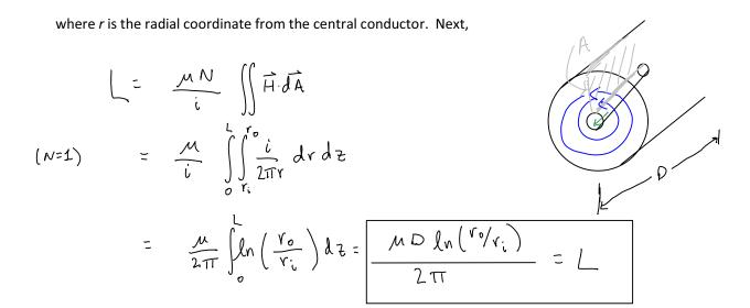
Let's compare with the square geometry. The bigger the depth, D, the larger the area over which flux crosses, and so the bigger the inductance, as before. But now, the other dimension of this area is linked to the path-length for the field lines, so that the growth in L is much slower (logarithmic) with an increase in this dimension ( $r_0$  relative to  $r_i$ ).
