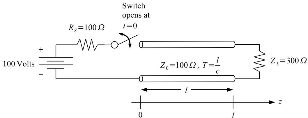
A transmission line of length  $l$ , characteristic impedance  $Z_0 = 100 \Omega$ , and one-way time of flight  $T = l/c$  is connected at  $z = 0$  to a 100 volt DC battery through a series source resistance  $R_s = 100 \Omega$  and a switch. The  $z = l$  end is loaded by a  $300 \Omega$  resistor.
