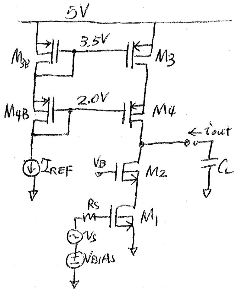
$\Rightarrow$  Need voltage source for  $V_B$ . Use diode connected NMOS (M2B) between  $I_{REF}$  and PMOS
