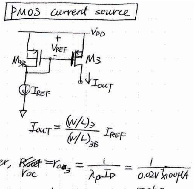
$\implies$  need to cascode circuit for current source. Add a current buffer (CG) for high  $R_{\text{out}}$ . Source resistance of current supply
