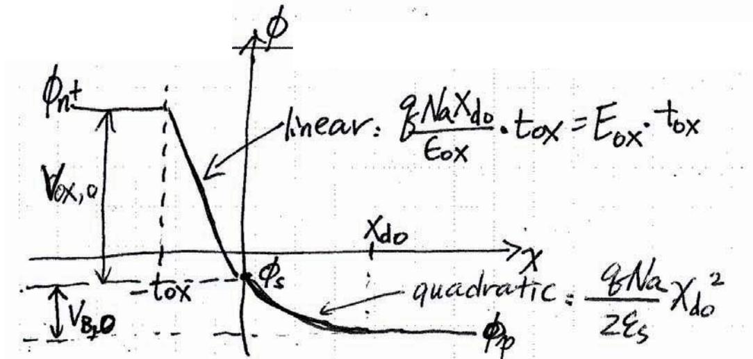
$V_{B,O}$  is potential drop across semiconductor *body*, while  $V_{ox,O}$  is potential drop across oxide. (Note that unit wise: potential, voltage and bias are the same).
