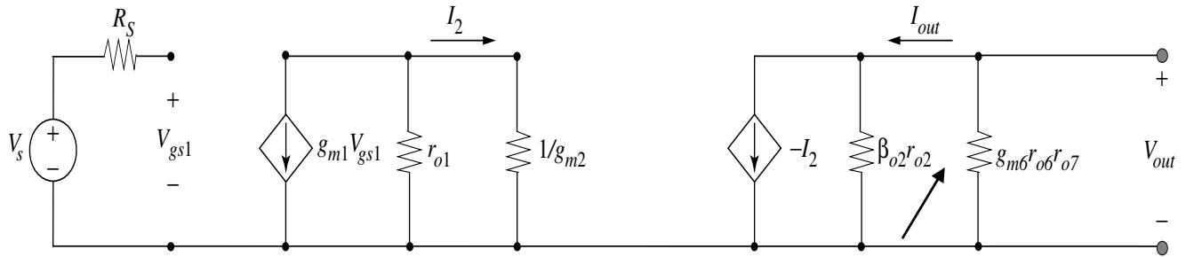
$$R_{out} = \beta_{o2} r_{o2} \| g_{m6} r_{o6} r_{o7}$$
