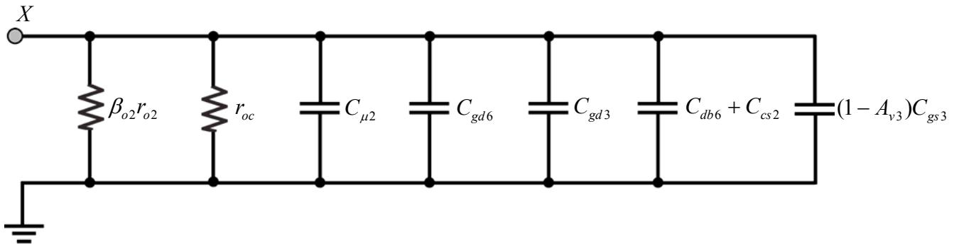
$$A_{vo} = \frac{V_{out2}}{V_s} = -g_{m1} (\beta_{o2}r_{o2} \| g_{m6}r_{o6}r_{o7}) \approx \frac{V_{out}}{V_s}$$
