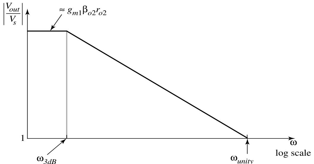
$$\omega_{3dB} = \sqrt{\frac{1}{(\beta_{o2} r_{o2} \| g_{m6} r_{o6} r_{o7})}}$$
