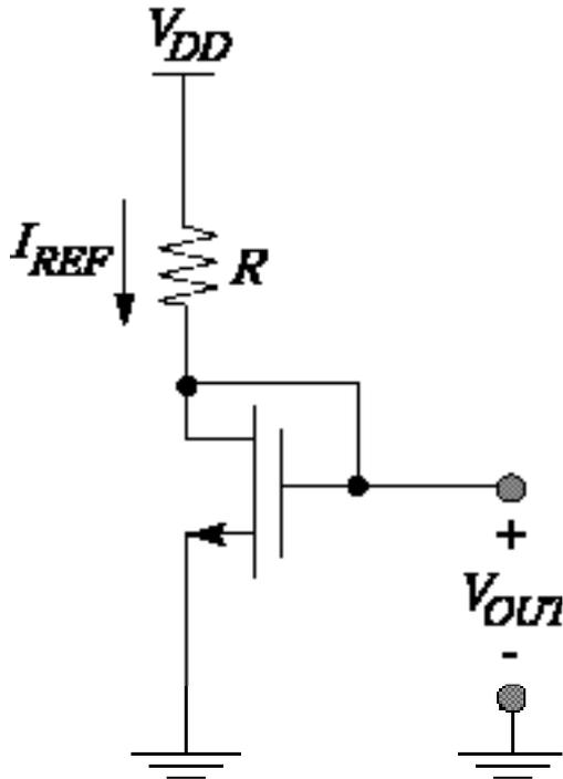
$$I_{REF} = \frac{V_{DD} - V_{OUT}}{R}$$
