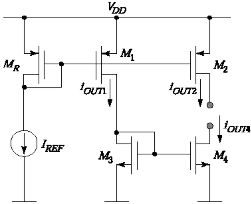
$$I_{OUT1} = I_{REF} \frac{\left(\frac{W}{L}\right)_1}{\left(\frac{W}{L}\right)_R} \quad I_{OUT2} = I_{REF} \frac{\left(\frac{W}{L}\right)_2}{\left(\frac{W}{L}\right)_R}$$
