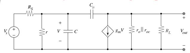
Replace voltage source and resistance with current source and resistance using Norton Equivalent
