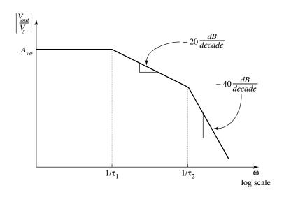
$$\tau_1 + \tau_2 = R'_{out}C_{\mu} + R'_{in}C_{\mu}(1 + g_m R'_{out}) + R'_{in}C_{\pi}$$
