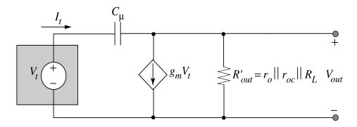
The input impedance  $Z_i$  is determined by applying a test voltage  $V_t$  to the input and measuring  $I_t$ :
