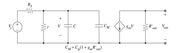
• The Miller capacitance is lumped together with  $C_{\pi}$ , which results in a single pole low pass filter at the input
