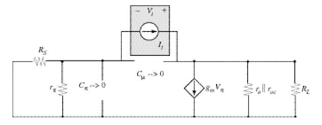
Let  $R'_{in} = R_S \parallel r_{\pi}$  and  $R'_{out} = r_o \parallel r_{oc} \parallel R_L$
