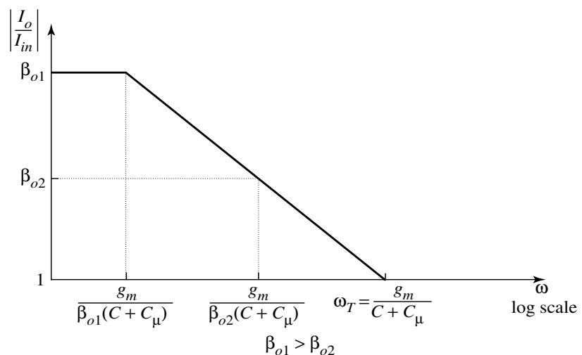
Examine how transistor parameters affect  $\omega_T$
