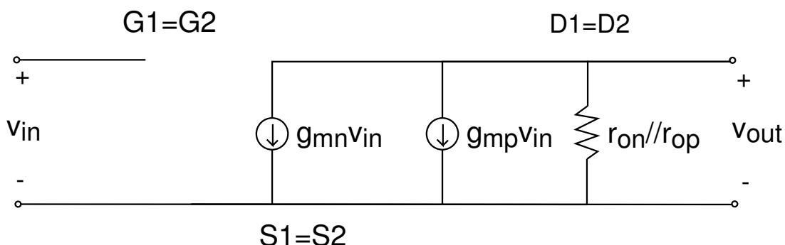
$$A_v = - \left( g_{mn} + g_{mp} \right) \left( r_{on} / \! / r_{op} \right)$$
