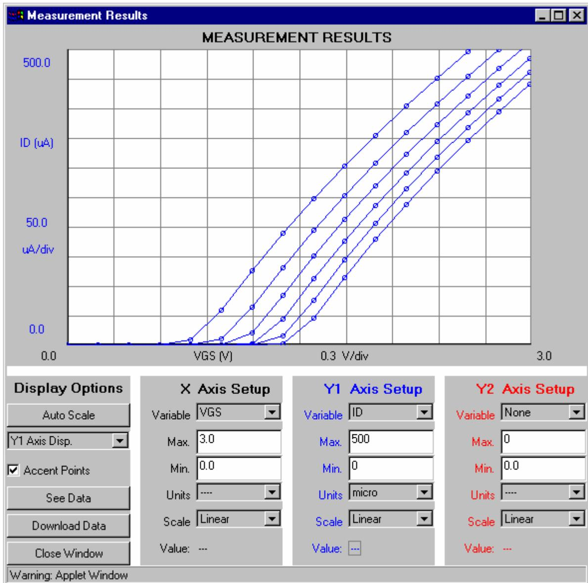
Triode Region  $V_{DS} \sim 0.1\text{V}$
