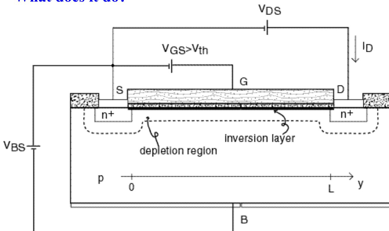
**Key Assumption (thus far):  $V_{BS} = 0 \Rightarrow V_{GS} = V_{GB}$**
