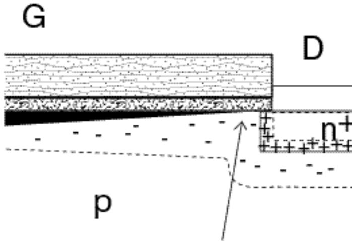
$$V(L) = V_{DSsat} = V_{GS} - V_T$$
