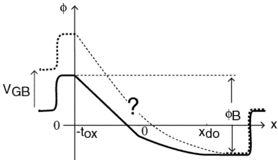
Oxide is an insulator  $\Rightarrow$  no current anywhere in structure
