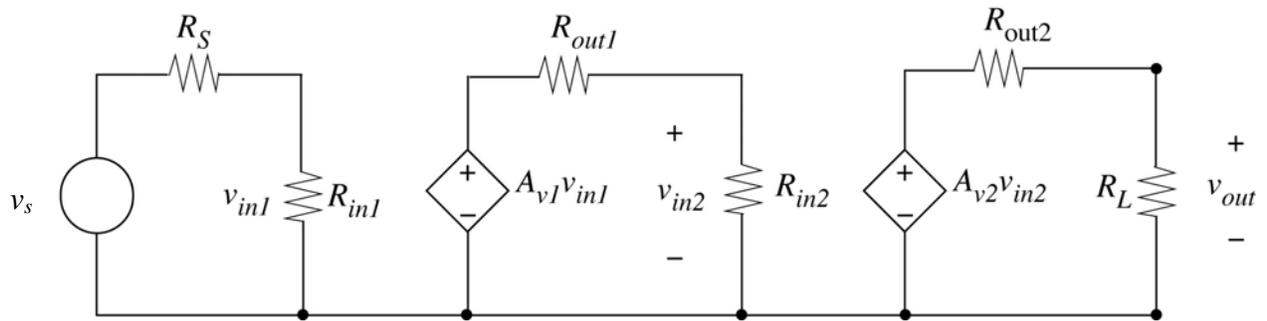
c) Calculate  $R_{in2}$ ,  $A_{v2}$ , and  $R_{out2}$ .
