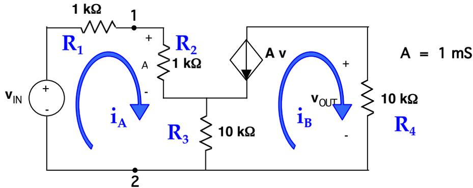
(a) What is the voltage  $v_{OUT}$  when the input voltage,  $v_{IN}$ , is 2 Volts?
