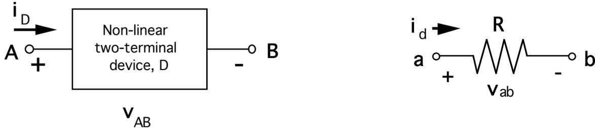
A linear equivalent circuit for the device D valid for small signal operation about a bias point,  $v_{AB} = V_{AB}$ , is shown to the right. What is R for the bias point  $V_{AB} = 2\text{V}$ ?
