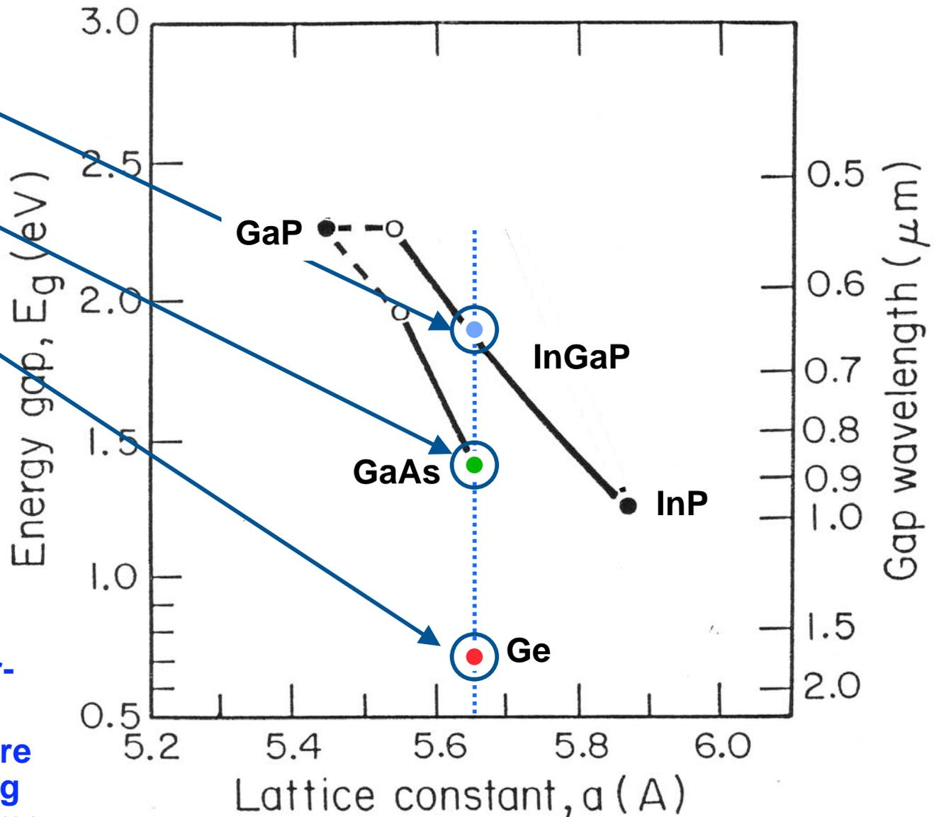
Multi-junction cells exceed 50% conversion efficiency. They are costly so are used in sun tracking concentrator systems.
