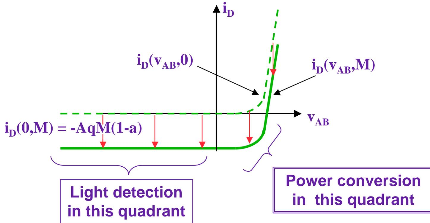
**Solar Cells:** A single band-gap diode misses much of the solar energy spectrum
