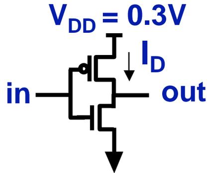
$$I_D = I_{S,s-t} e^{\frac{v_{GS} - V_T}{nV_t}} \left( 1 - e^{-\frac{v_{DS}}{V_t}} \right)$$
