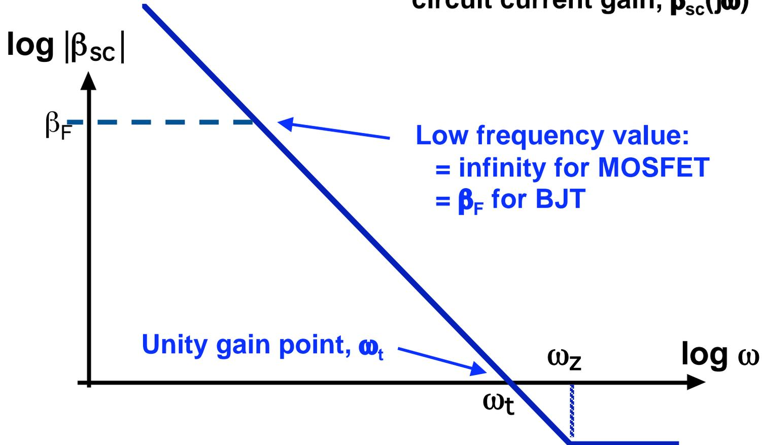
$$\omega_t \approx \left\{ \begin{array}{ll} g_m / C_{gs} = 3\mu_{Ch} (V_{GS} - V_T) / 2L^2 = 3s_{Ch} / 2L & \text{MOSFET, no vel. sat.} \\ g_m / C_{gs} = W s_{sat} C_{ox}^* / W L C_{ox}^* = s_{sat} / L & \text{MOSFET, w. vel. sat.} \\ g_m / (C_\pi + C_\mu) \Rightarrow \lim_{I_C \rightarrow \infty} \approx 2D_{min,B} / w_B^2 & \text{BJT, large } I_C \end{array} \right\} = \frac{1}{\tau_{tr}}$$
