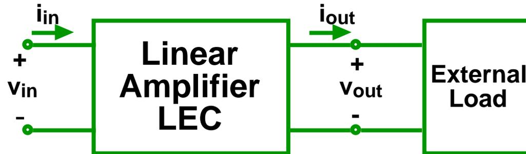
The typical linear amplifier is comprised of multiple building-block stages, often such as the single transistor stages we introduced on Slide 14 (and which will be the topic of Lect. 19):
