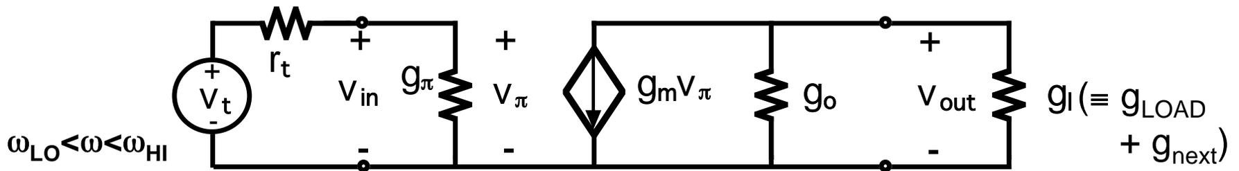
Valid for  $\omega_{LO} < \omega < \omega_{HI}$ , the "mid-band" range, where all bias capacitors are shorts and all device capacitors are open.
