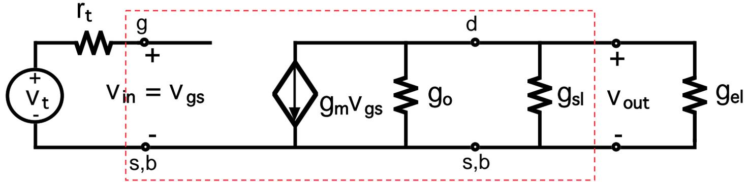
$$V_{out} = -\frac{g_m V_{in}}{g_o + g_{sl} + g_{el}} = -\frac{g_m V_t}{g_o + g_{sl} + g_{el}}$$
