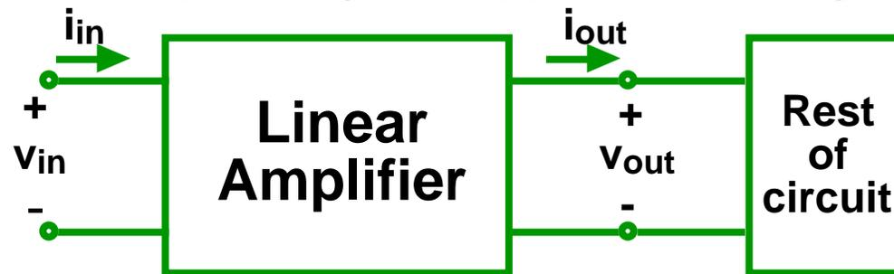
Voltage gain,  $A_v = v_{out}/v_{in}$
