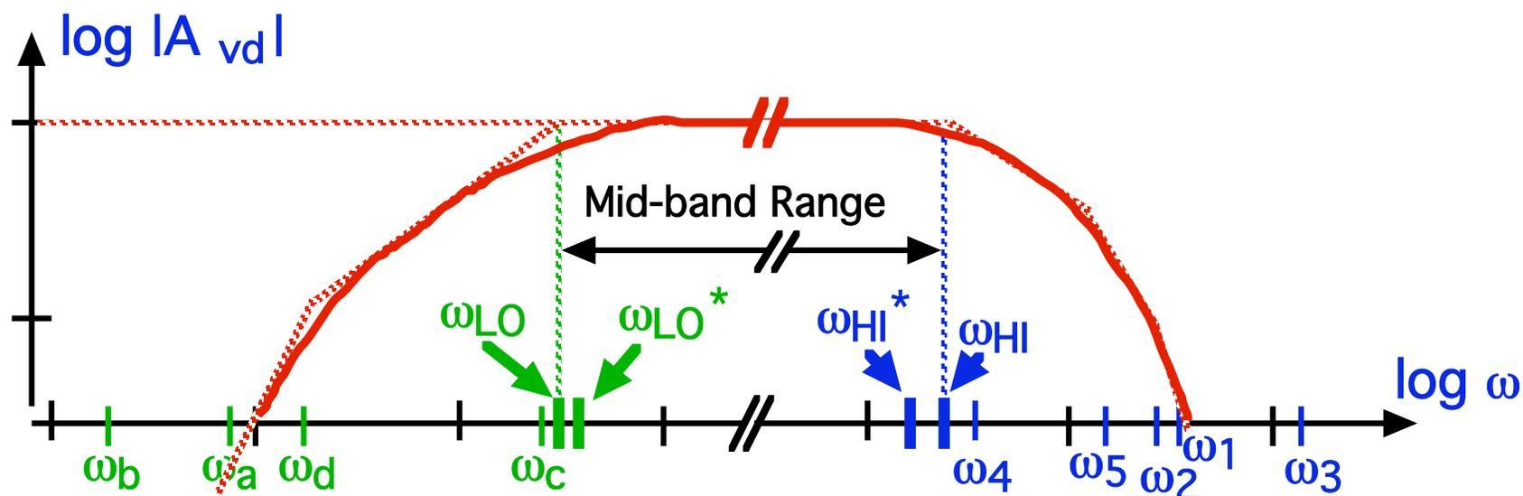
All of the parasitic and intrinsic device capacitances are effectively open circuits
