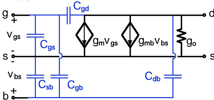
$$g_m = K[V_{GS} - V_T(V_{BS})][1 + \lambda V_{DS}] \approx \sqrt{2KI_D}$$
