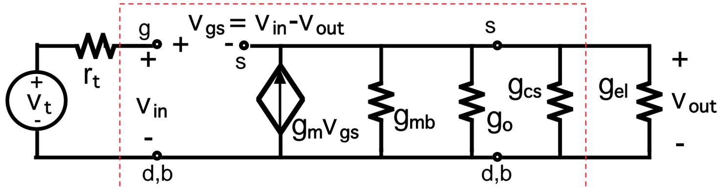
$$v_{out} = \frac{g_m (v_{in} - v_{out})}{g_{mb} + g_o + g_{cs} + g_{el}} \Rightarrow v_{out} = \frac{g_m v_{in}}{g_m + g_{mb} + g_o + g_{cs} + g_{el}} \approx \frac{g_m v_{in}}{g_m + g_{mb}} = \frac{v_{in}}{1 + \eta}$$
