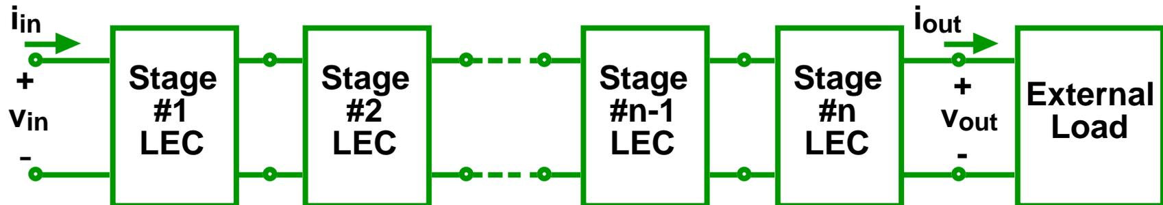
A useful concept and tool for analyzing, as well as designing, such multi-stage amplifiers is the two-port representation.
