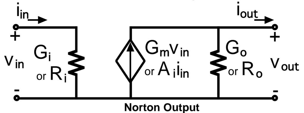
Two-ports can simplify the analysis and design of multi-stage amplifiers:
