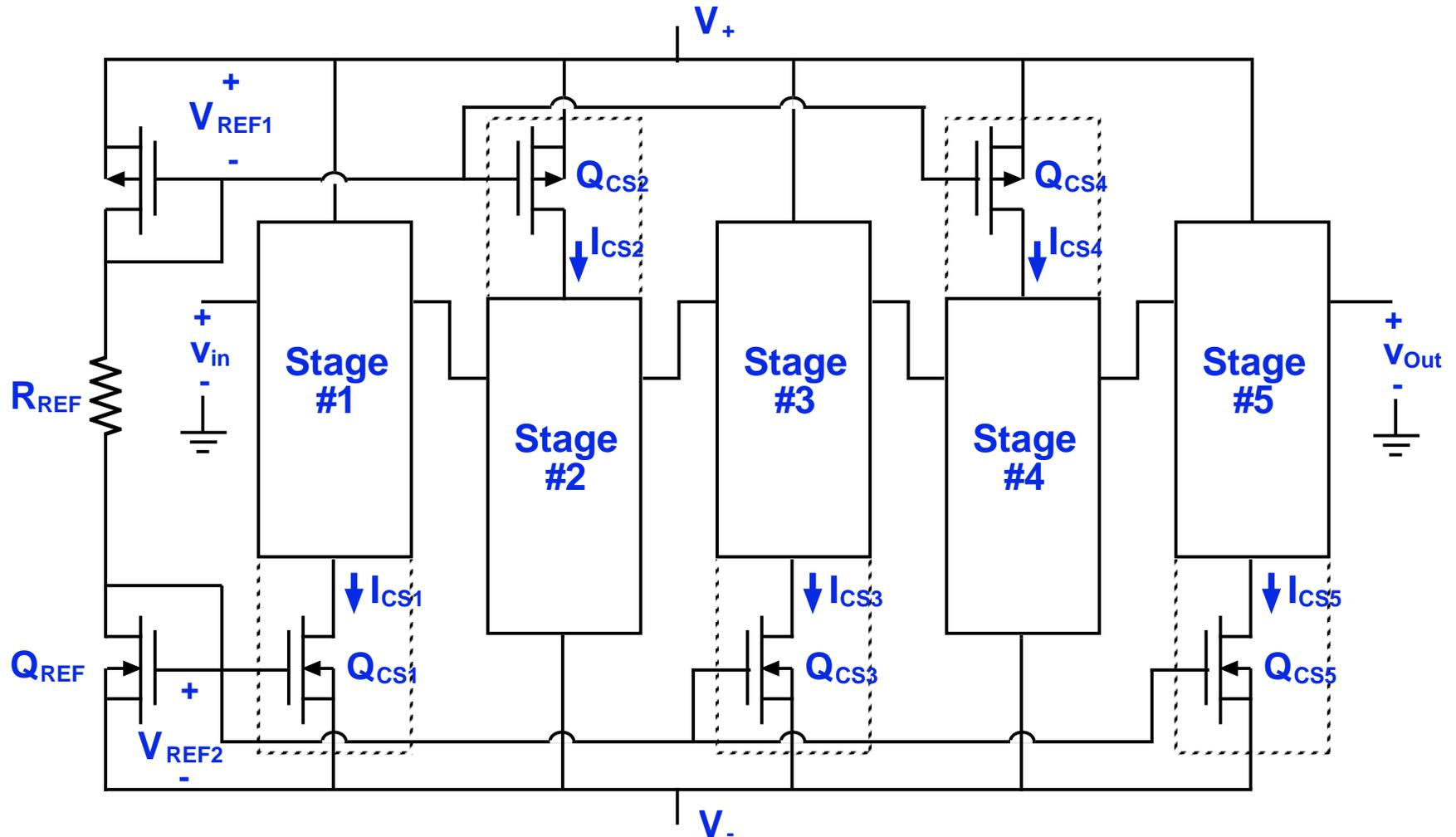
⇒ The current mirror voltage reference method can be extended to bias multiple stages, and one reference chain can be used to provide  $V_{REF}$  to all the sources and sinks in an amplifier.
