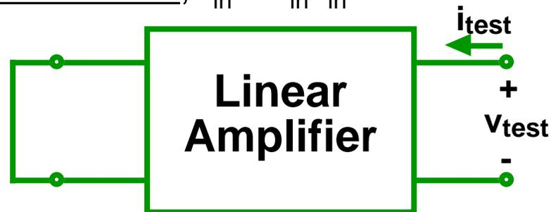
Output resistance,  $r_{out} = v_{test}/i_{test}$  with  $v_{in} = 0$
