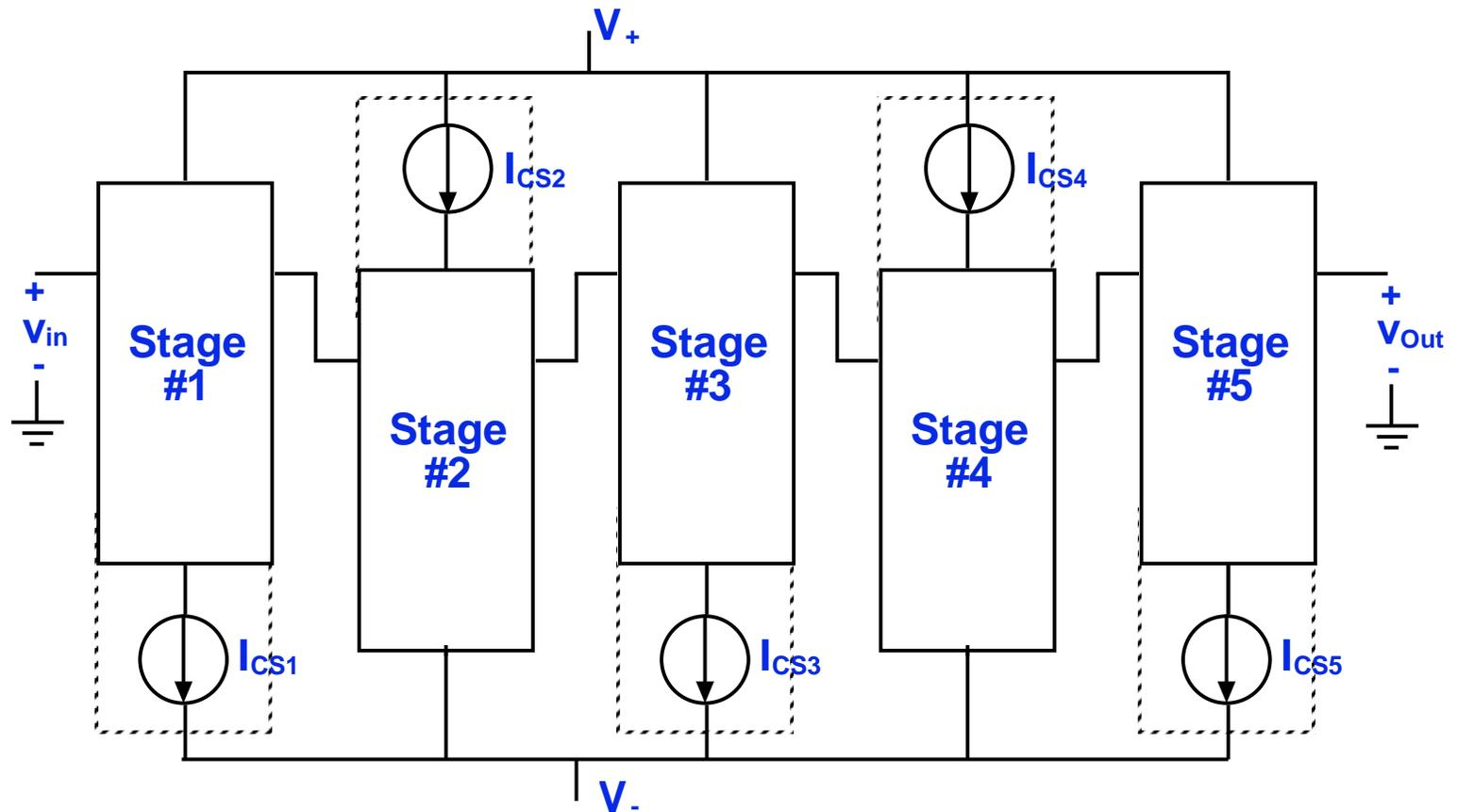
When looking at a complex circuit schematic it is useful to identify the voltage reference chain and the biasing transistors and replace them all by current source symbols. This can reduce the apparent complexity dramatically.
