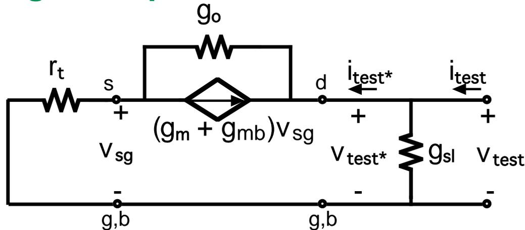
**Output resistance** - Set  $v_t = 0$ , and apply  $v_{test^*}$  to output; find  $i_{test^*}$ :
