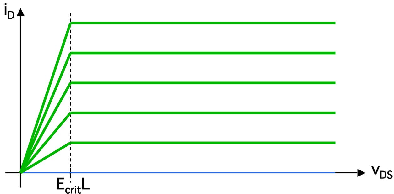
Note first that in the forward active region where  $v_{DS} \geq E_{crit} L$ , the curves in the output family are evenly spaced, indicating a constant  $g_m$ :
