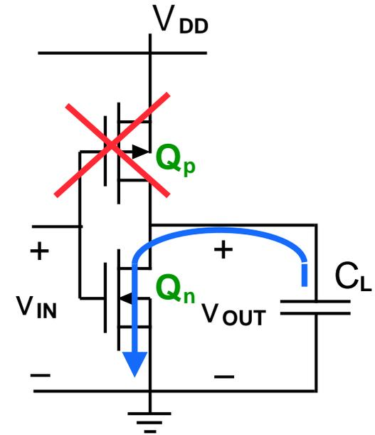
Minimum cycle time:  $v_{IN}$ : LO to HI to LO;  $v_{OUT}$ : HI to LO to HI
