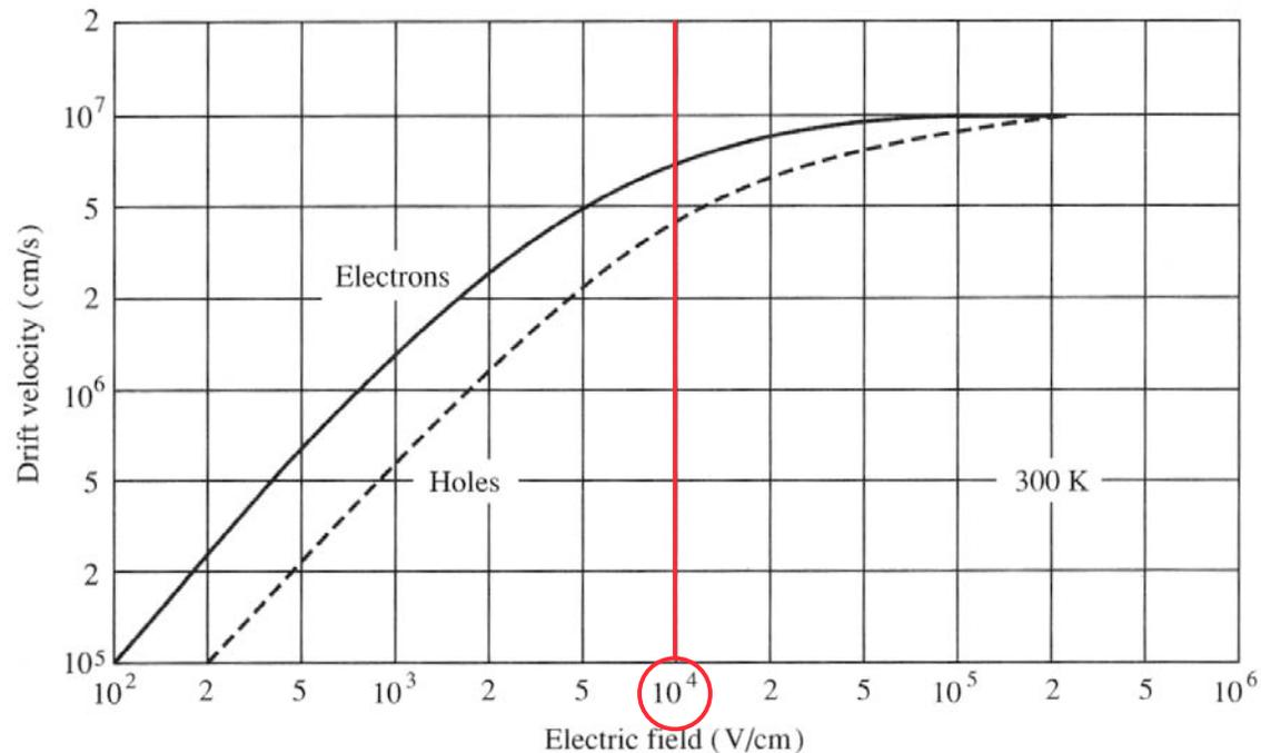
Clearly the velocity of the electrons and holes in the channel will be saturated at even low values of  $v_{DS}$ !
