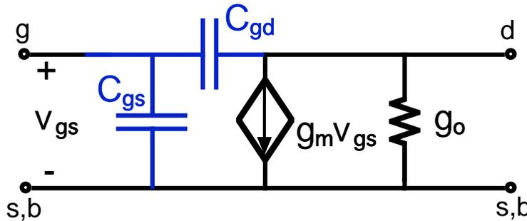
$$g_m \equiv \left. \frac{\partial i_D}{\partial v_{GS}} \right|_Q = W s_{sat} C_{ox}^*$$
