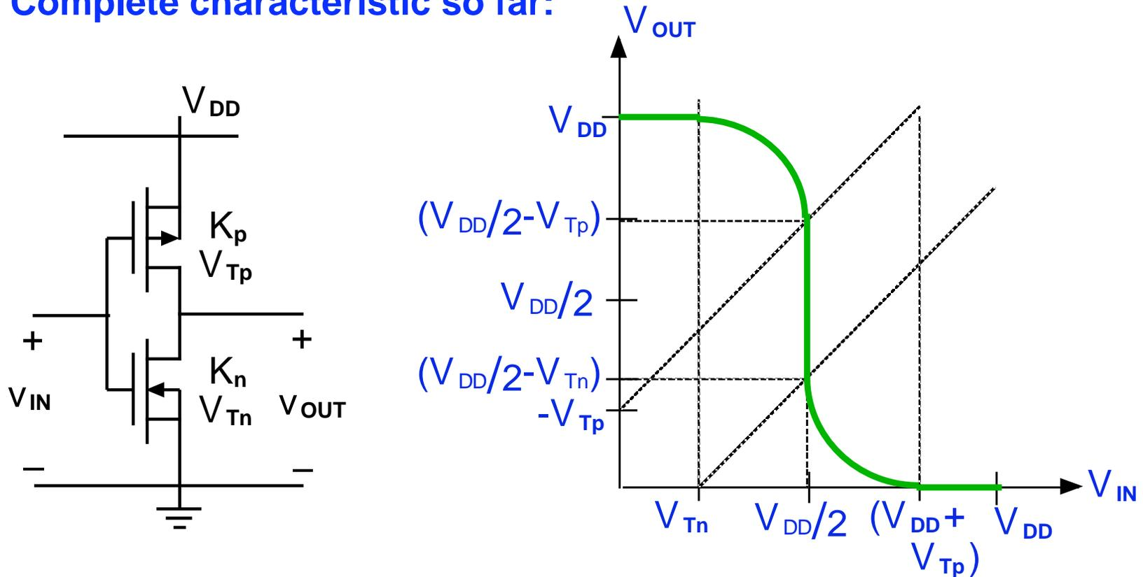
**NOTE:** We design CMOS inverters to have  $K_n = K_p$  and  $V_{Tn} = -V_{Tp}$  to obtain the optimum symmetrical characteristic.
