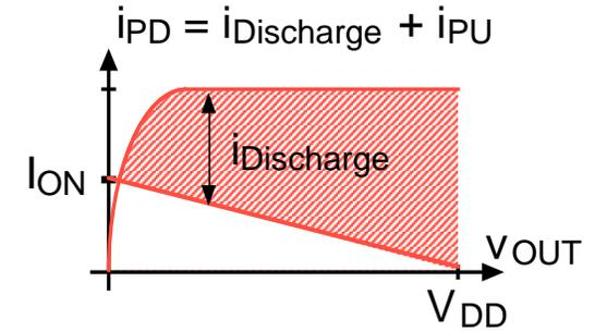
E-mode pull-up ( $V_{DD}$  on gate)
