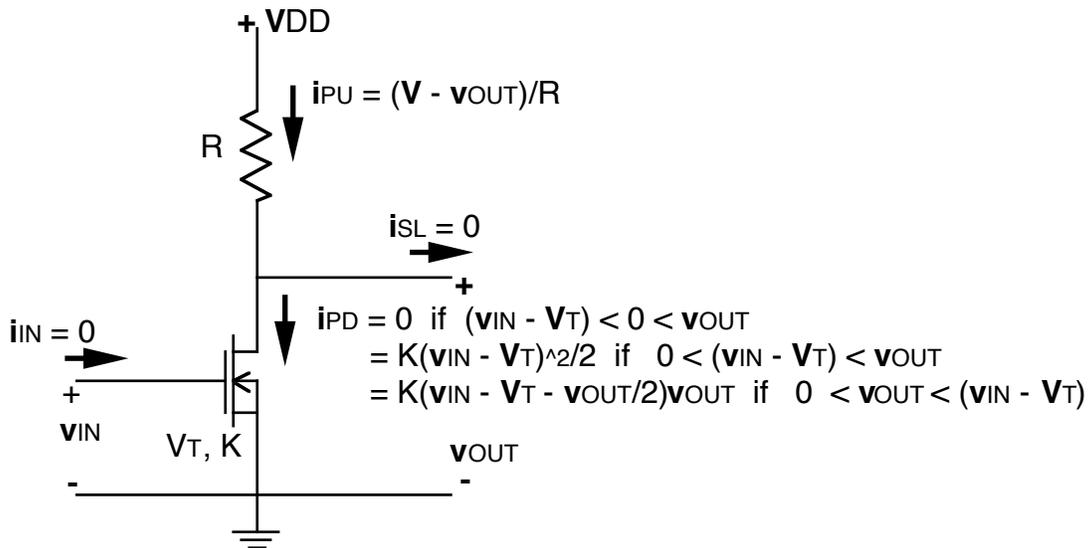
A MOSFET inverter with an n-channel MOSFET pull-down and resistor pull-up.
