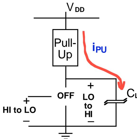
**Charging cycle:**  $i_{\text{Charge}} = i_{\text{PU}}$
