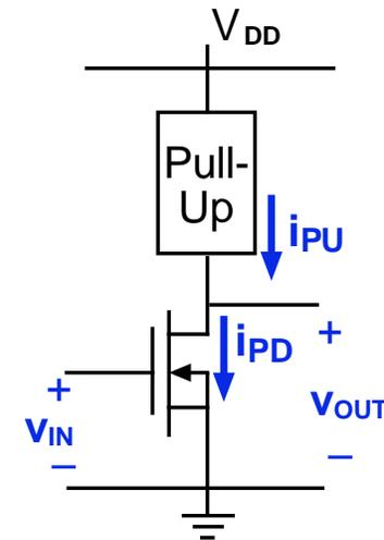
$$P_{Static,on} = I_{PU,on} V_{DD}$$
