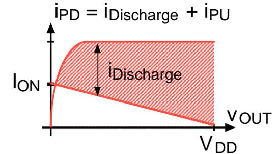
E-mode pull-up ( $V_{DD}$  on gate)
