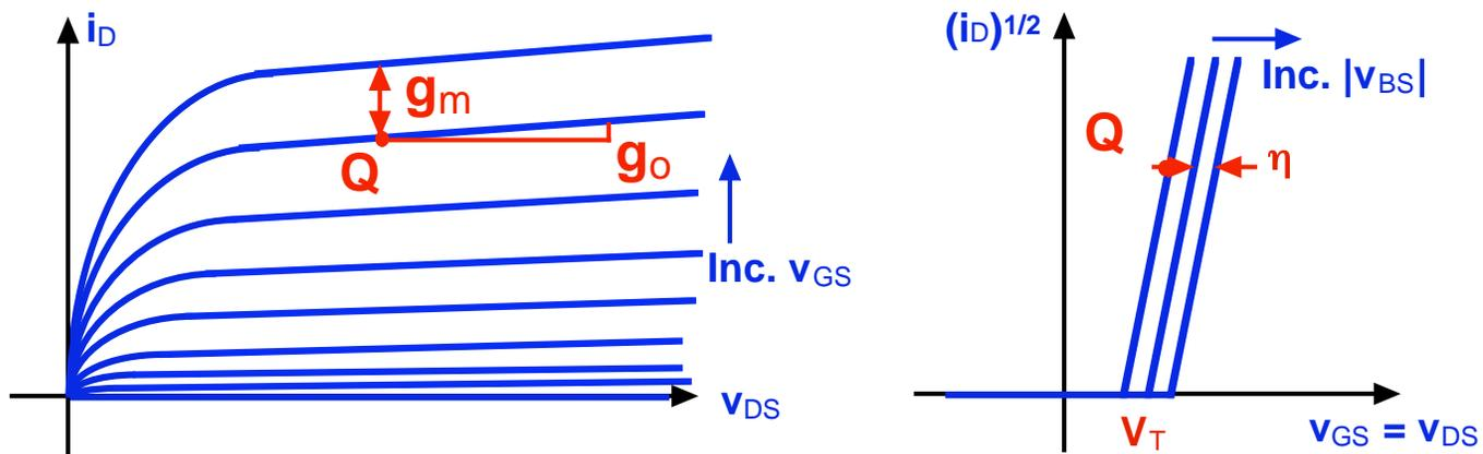
$$g_m = di_D/dv_{GS}|_Q; g_{mb} = \eta g_m \text{ with } \eta = -dV_T/dv_{BS}|_Q; g_o = di_D/dv_{DS}|_Q$$
