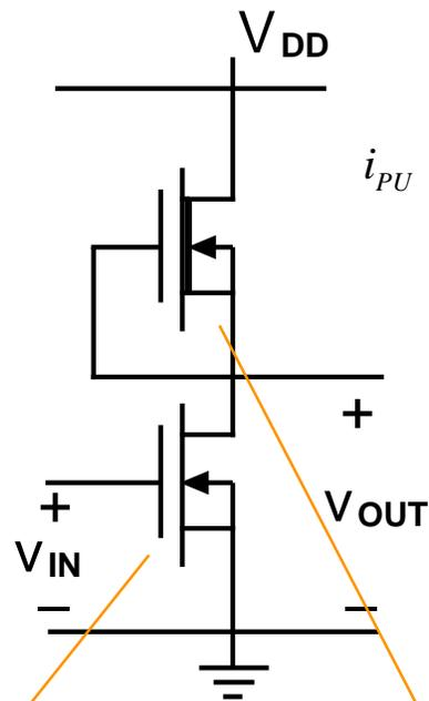
$$i_{PU} = \begin{cases} K_{PU} |V_{T,PU}|^2 / 2 & \text{when } 0 < |V_{T,PU}| < [V_{DD} - v_{OUT}] \\ K_{PU} [|V_{T,PU}| - (V_{DD} - v_{OUT}) / 2] (V_{DD} - v_{OUT}) & \text{when } 0 < [V_{DD} - v_{OUT}] < |V_{T,PU}| \end{cases}$$
