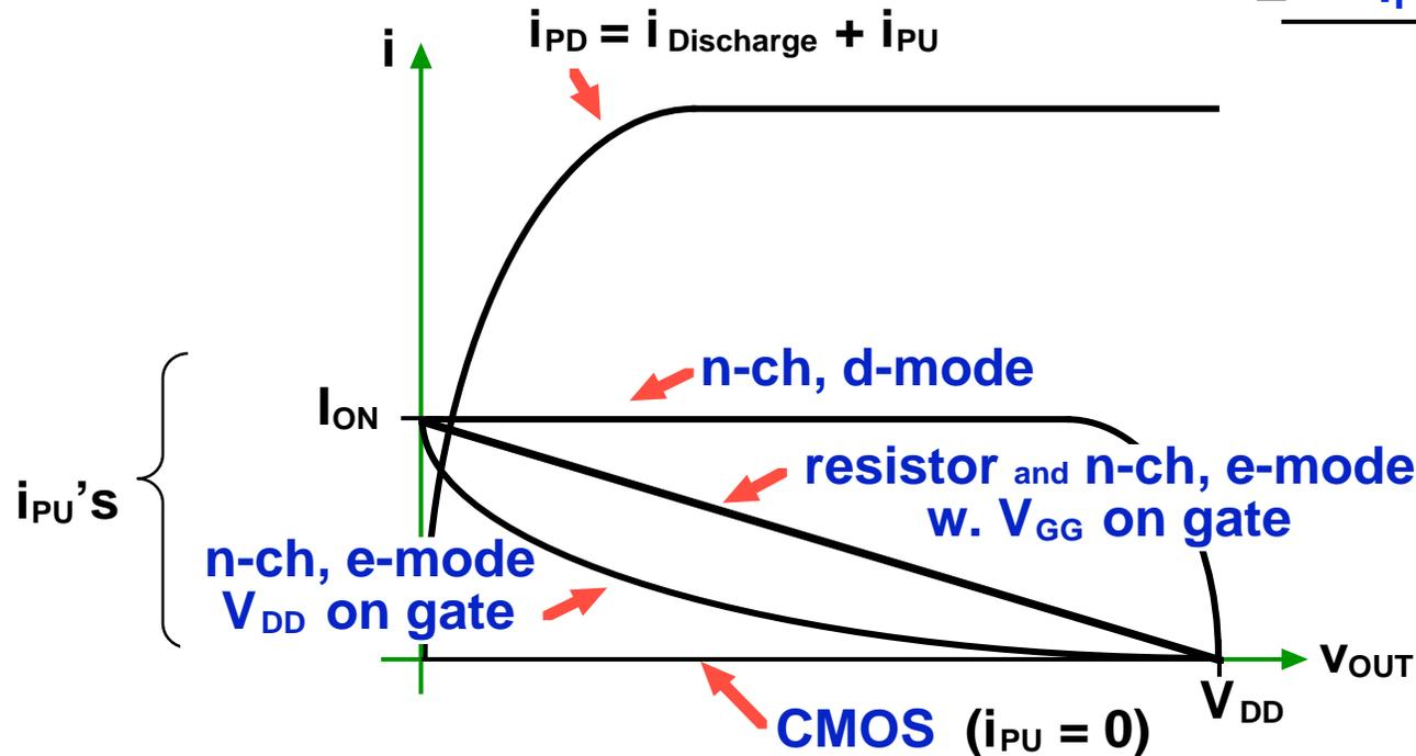
✓ The discharge current ( $i_{Discharge}$ ) is the difference between the upper curve ( $i_{PD}$ ) and the appropriate lower curve ( $i_{PU}$ ).
