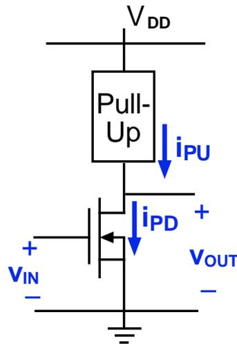
$$P_{Static,off} = I_{PD,off} V_{DD} \quad (\approx 0)$$
