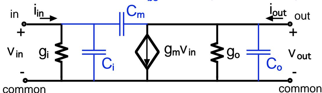
Most linear circuits are designed to operate at frequencies where the capacitors look like open circuits. We can thus do our designs neglecting them.\*
