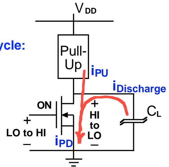
$$\frac{1}{2} C_L V_{DD}^2 \text{ Dissipated, } \frac{1}{2} C_L V_{DD}^2 \text{ Stored}$$
