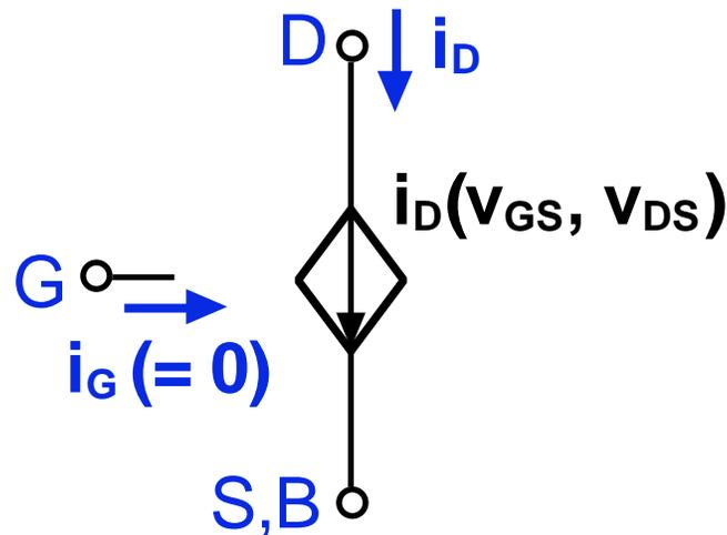
$$i_{G,s-t}(v_{GS}, v_{DS}, v_{BS}) = 0$$
