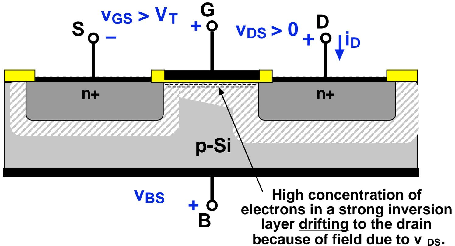
**n-type surface channel; drift flux from source to drain**
