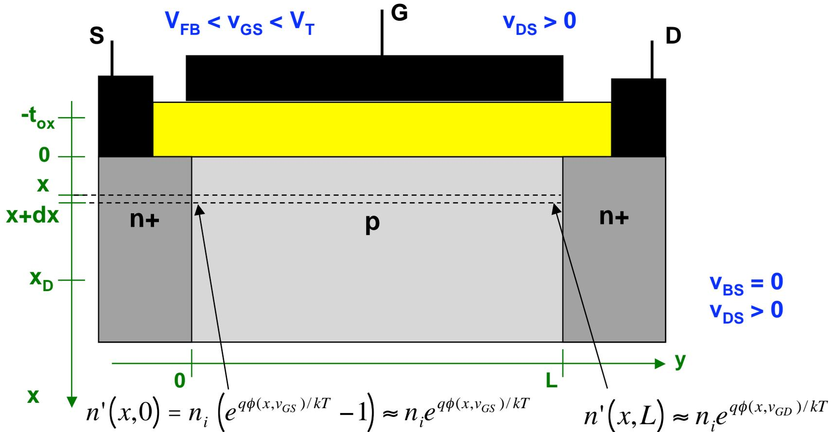
$$di_D(x) = qD_e \frac{n'(x,0) - n'(x,L)}{L} W dx \approx \frac{W}{L} D_e q n_i e^{q\phi(x,v_{GS})/kT} \left( 1 - e^{-qv_{DS}/kT} \right) dx$$
