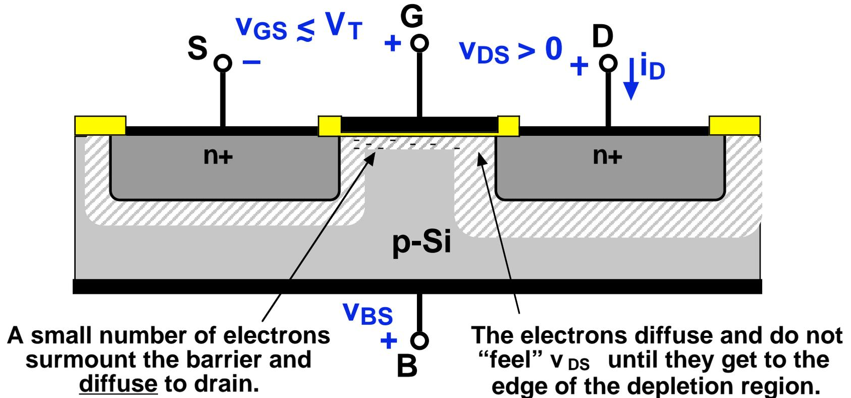
No surface channel; diffusion flux from source to drain when  $v_{DS} > 0$
