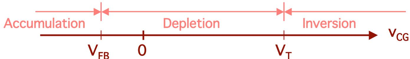
Inversion layer sheet charge density:  $q_N^* = -C_{ox}^* [v_{GC} - V_T(v_{BC})]$
