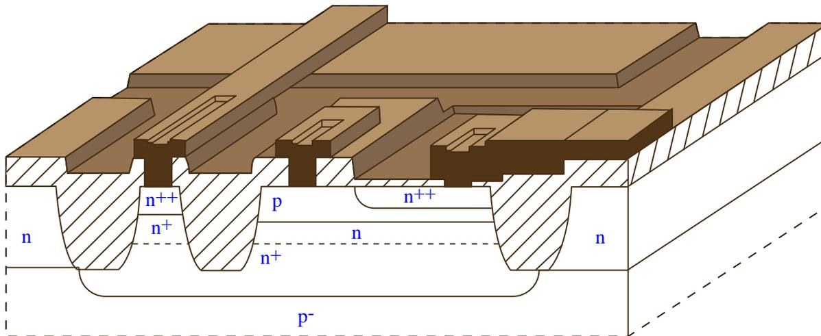
**Oxide isolated integrated BJT - a modern process**
