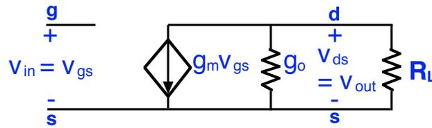
We find  $g_m = 1.5 \times 10^{-6}$  mho and  $g_o = 1.1 \times 10^{-6}$  mho, and using the  $R_L$  above we have  $1/R_L = G_L = 1.1 \times 10^{-6}$  mho. Thus,  $A_v = v_{out}/v_{in} = -g_m/(g_o + G_L) \approx -0.7$ .
