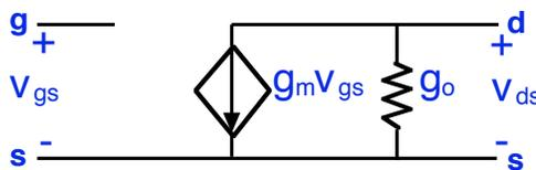
with  $g_m = (W/L) \mu_e C_{ox}^* V_{DS}$  and  $g_o = (W/L) \mu_e (C_{ox}^* V_{GS} + \alpha)$
