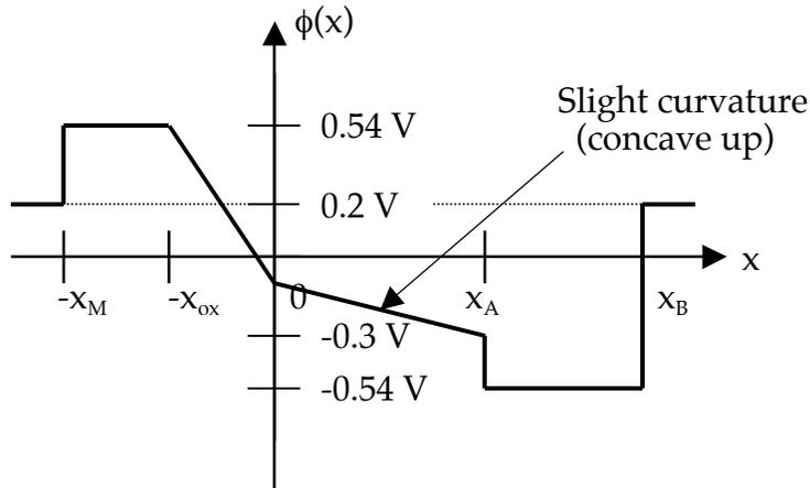
c)  $x_p = x_A = (2 \epsilon_{Si} \Delta\phi / q N_A)^{1/2} = 10 \text{ nm}$ . We find  $\Delta\phi = 0.08 \text{ V}$
