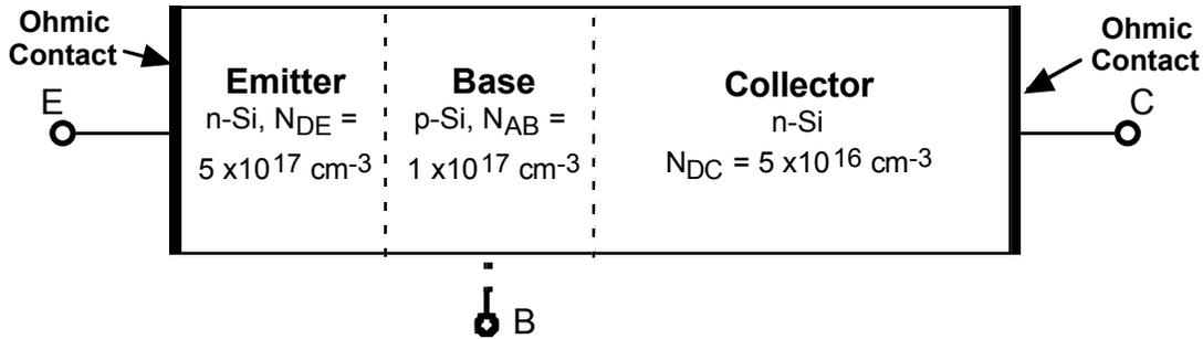
i) On the axes provided, sketch and label the excess minority carrier profiles when both junctions are forward biased with  $v_{BE} = v_{BC} = 0.6$  V. Notice that this is not a bias in the forward active region.
