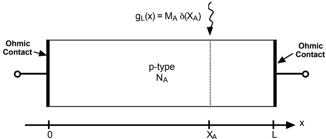
The general equation governing the excess minority carriers in a uniformly doped material is
