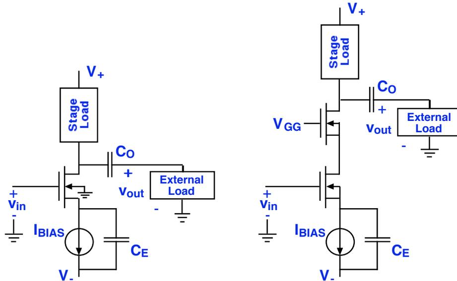
Use the two-port models for the common-source and common-gate stages (shown below) to compare the voltage gain and output resistance of this two-stage amplifier to the single common-source amplifier shown above on the left.
