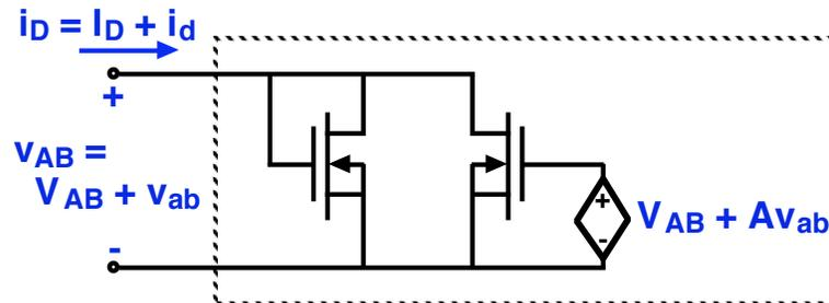
The two n-MOS transistors in this circuit are identical with the same dimensions and values of  $K$ ,  $V_T$ , and  $\lambda$ . Assume that  $V_{AB} > V_T$  so both transistors are active (and operating in saturation).
