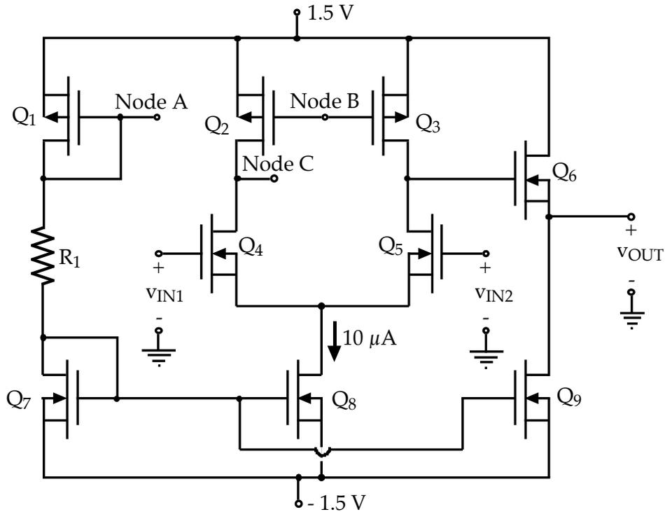
The drain current of  $Q_8$  is known to be  $10 \mu\text{A}$ , and  $W_7$ , the width of  $Q_7$ , is known to be  $W_{\min}$ . The resistor  $R_1$  has been selected so that  $Q_1$  and  $Q_7$  are biased with  $|V_{GS} - V_T| = 0.1 \text{ V}$ . The widths of  $Q_2$ ,  $Q_3$ ,  $Q_4$ , and  $Q_5$  have been chosen so that for each of them  $|V_{GS} - V_T| = 0.1 \text{ V}$  when  $v_{IN1} = v_{IN2} = 0$ .
