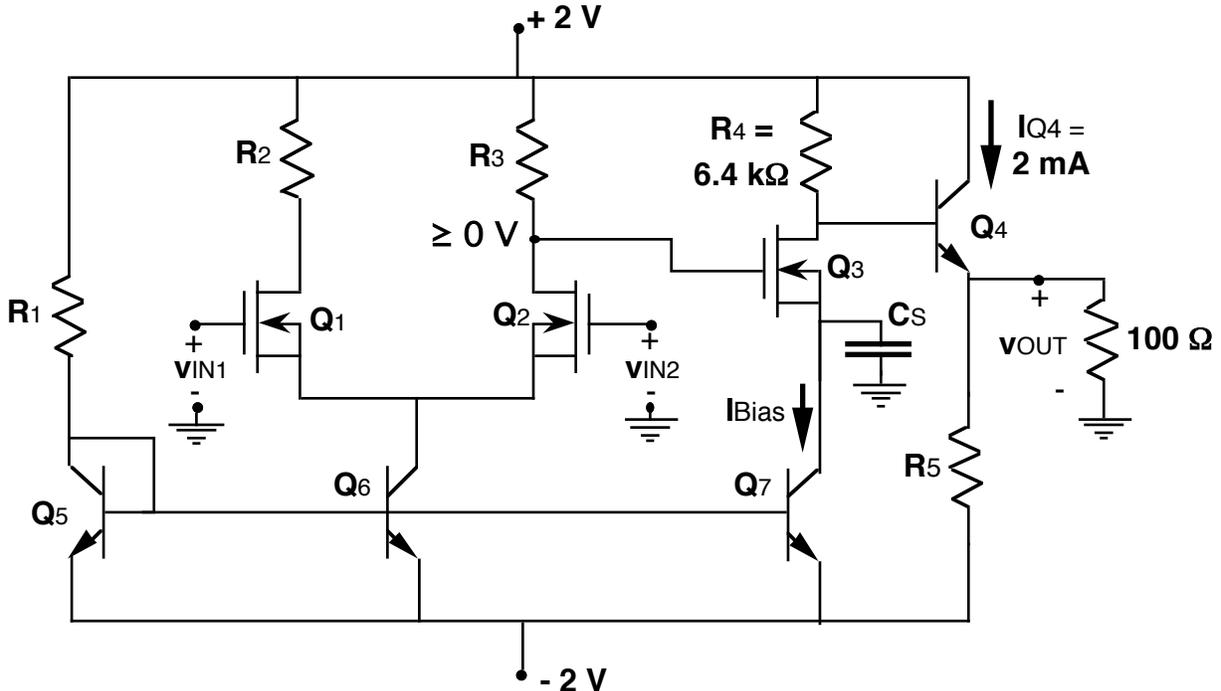
Note that value of the resistor  $R_4$ , the quiescent collector current on  $Q_4$ , and minimum quiescent voltage on the gate of  $Q_3$  are indicated on the schematic, as are the supply voltages.
