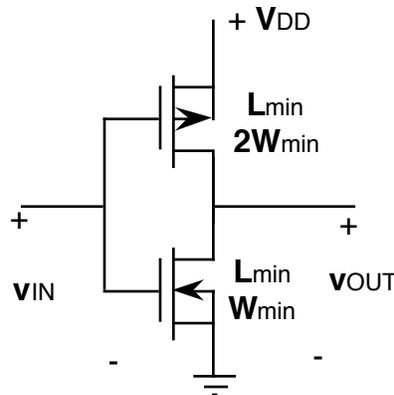
This minimum size inverter is shown above. The gate delay,  $\tau_{GD}$ , of this minimum size inverter is found to be 100 ps ( $10^{-10}$  s) when the fan-out is one. We will call this gate delay the minimum gate delay,  $\tau_{min}$ .
