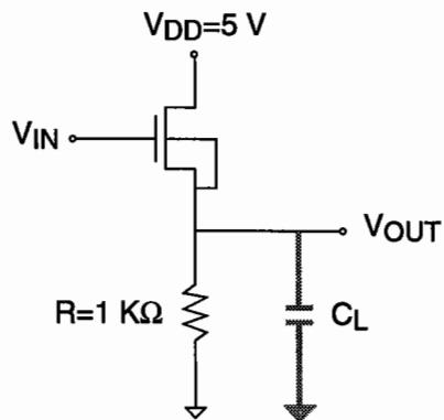
The parameters of the transistor are:  $\mu_n C_{ox} = 50 \mu\text{A}/\text{V}^2$ ,  $W/L = 5$ , and  $V_T = 1 \text{ V}$ . Neglect channel length modulation in this problem.
