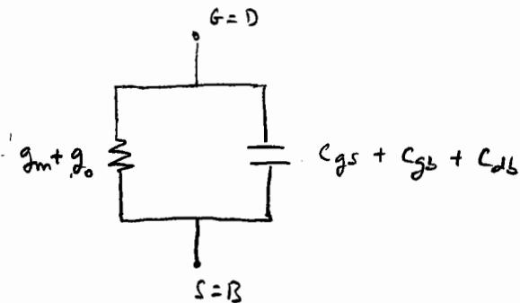
4. (15 points) An NMOS inverter with a resistor pull up was miswired and ended up as sketched below.
