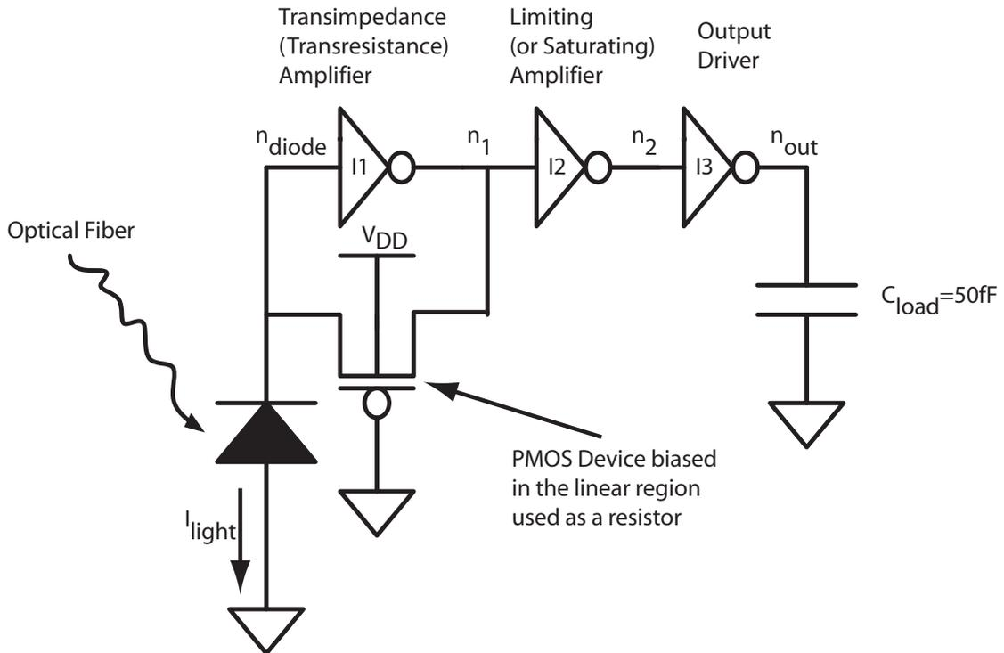
Figure 2: Schematic of optical receiver.
