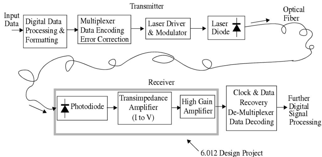
Figure 1: Block diagram of an optical transmitter and receiver.
