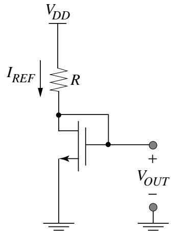
$$I_{REF} = \frac{V_{DD} - V_{OUT}}{R}$$
