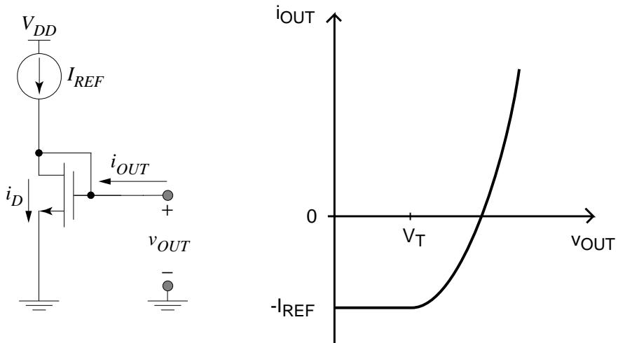
$V_{GS} = V_{DS}$  takes value needed to sink current:
