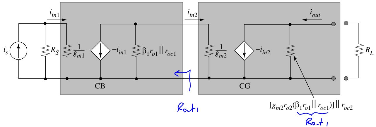
$$R_{out} = R_{out2} = r_{oc2} // [r_{o2}(1 + g_{m2}R_{out1})]$$
