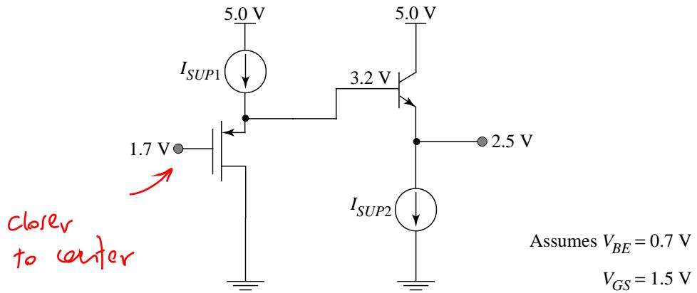
Trade-off:  $g_m(\text{PMOS}) < g_m(\text{NMOS}) \rightarrow \text{higher } R_{out}$
